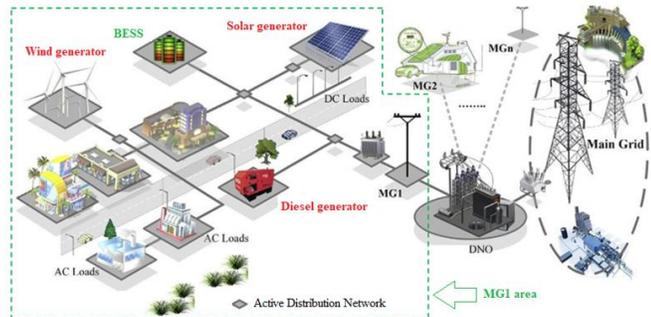
**Figure 1:** Micro Grid (MG) System Components [10].
