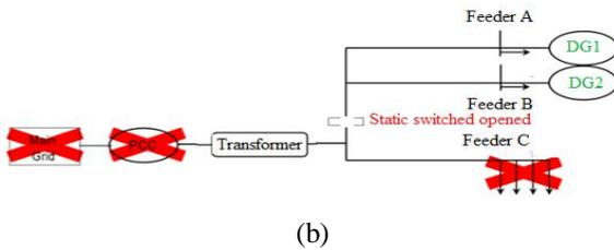
Figure 7: (a) Grid-connected mode [59], (b) Stand -alone mode [50]
