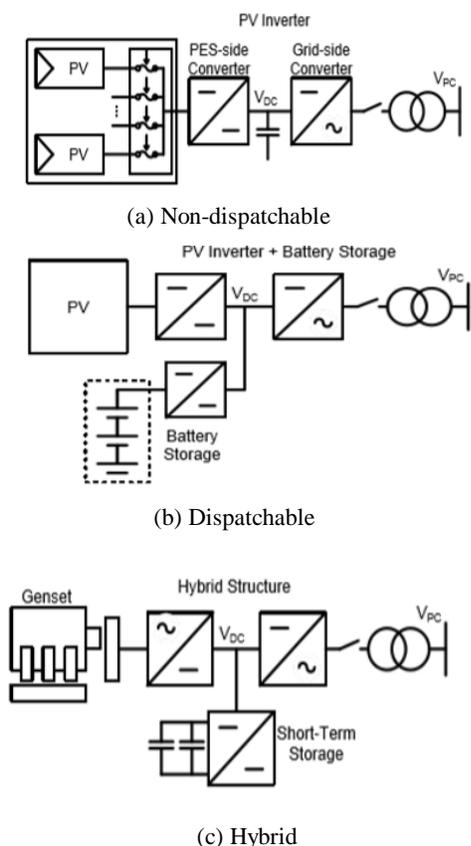
Figure 6: Power Flow Control Configuration in MG System [31]
