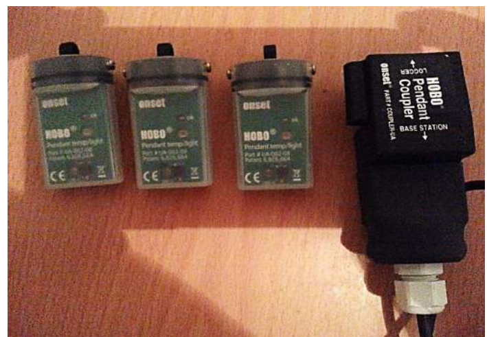
Fig. 1. Data-logger and three light meters used in the experiment.
