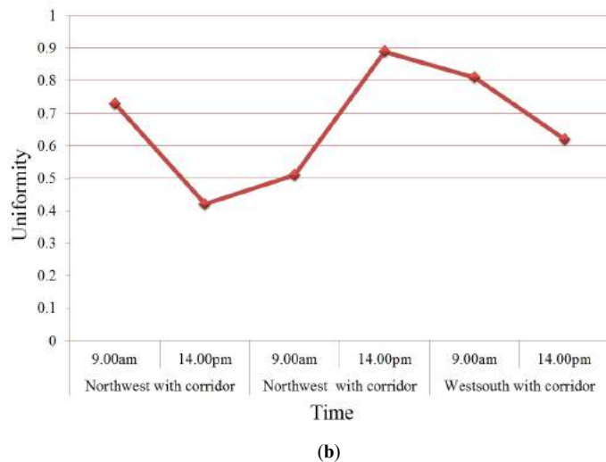
Fig. A1. The uniformity of daylight in both typology (bilateral and clerestory lighting) in different orientations at solstice (a) summer and (b) winter.
