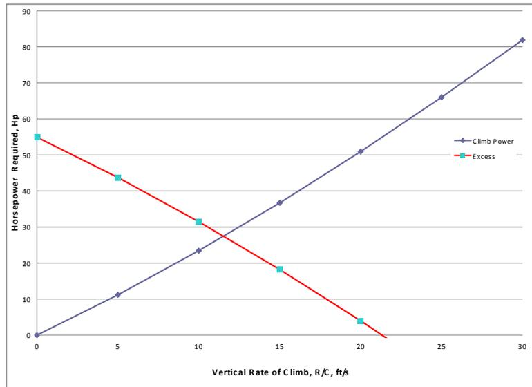
Figure 7: Graph Power Required Versus Climb Rate
