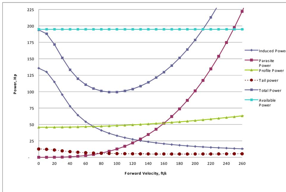
Figure 5: Power Required for Forward Flight versus Velocity
