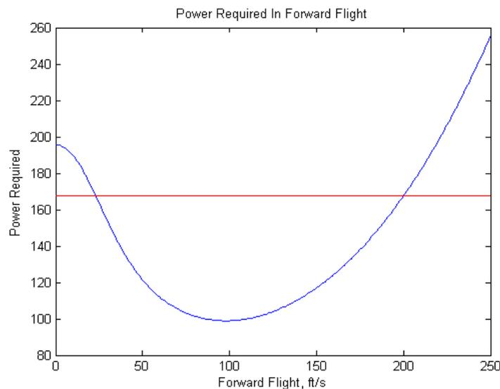
Figure 8: Forward Flight Power Graph plotted from Matlab
