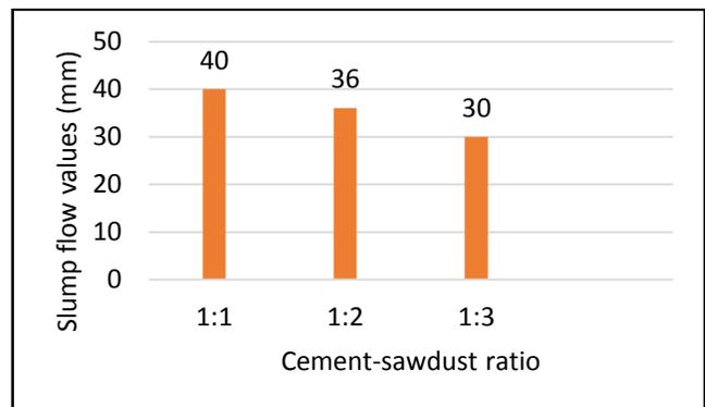
Figure 4 Slump flow values of sawdust concrete
