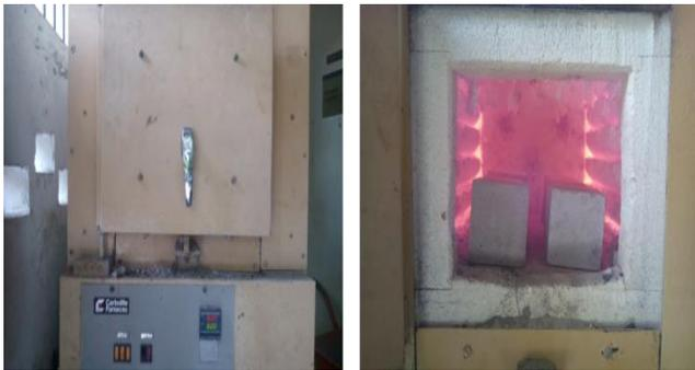
Figure 2 Electric furnace showing concrete specimens
