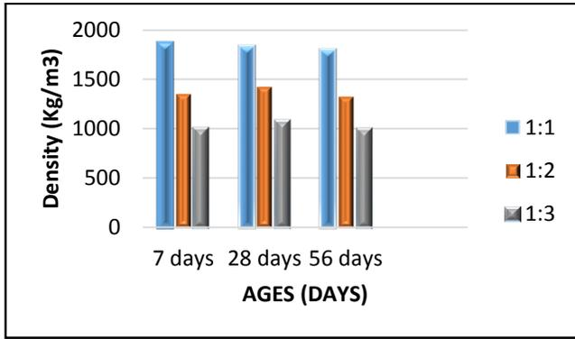
Figure 5 Density of 1:1, 1:2 and 1:3 sawdust concrete at 7, 28 and 56 days
