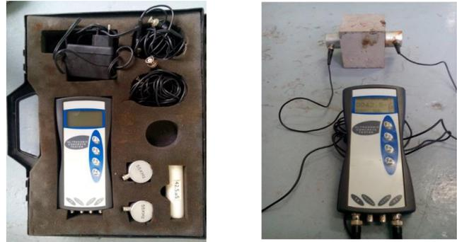
Figure 3 Ultrasonic pulse velocity (UPV) testing apparatus
