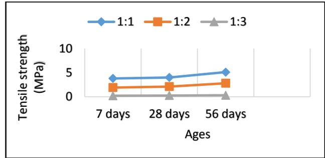
Figure 7 Split tensile strength of sawdust concrete
