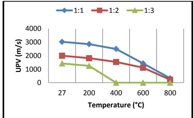
Figure 13 Average UPV values for sawdust concrete
