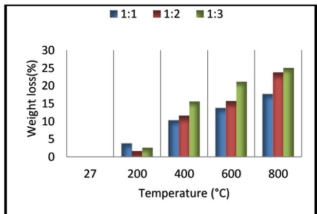
Figure 14 Weight loss of sawdust at elevated temperature
