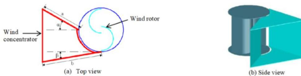
Figure 1. The design of wind concentrator [6]
