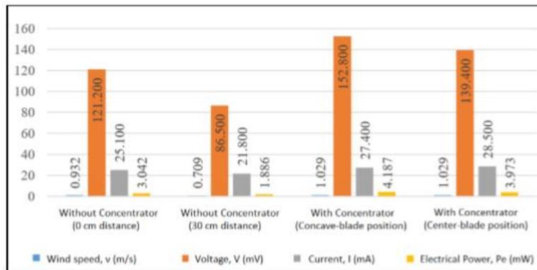
Figure 6. Generated voltage, current and electrical power at different conditions
