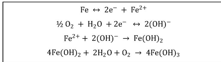
Figure 1.1 Electrochemical corrosion process
