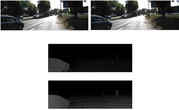
Figure 7. Up: The left camera image, the right camera image The LIDAR (ground Truth) Predicted Disparity map by the proposed method
