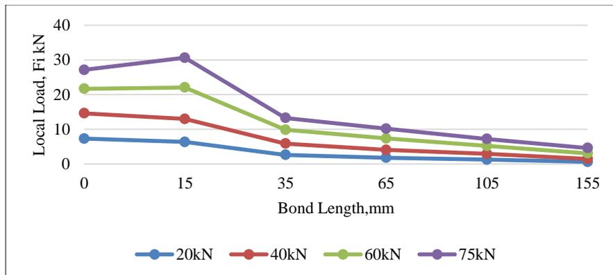
Figure 19: Local Load versus Bond Length for SPECS-7
