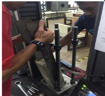
Figure 15: Installation of pull-out test rig
