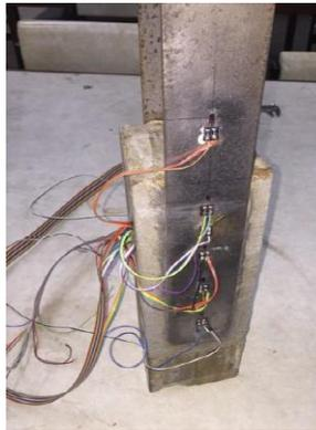
Figure 13: Sample SPECS-7 after installation of strain gauges
