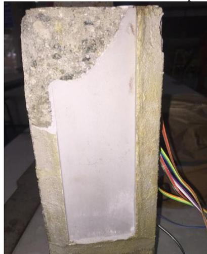
Figure 28: Concrete from SPECS-7 after failure
