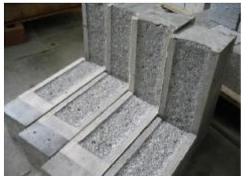
Figure 4: Readily hacked concrete surface
