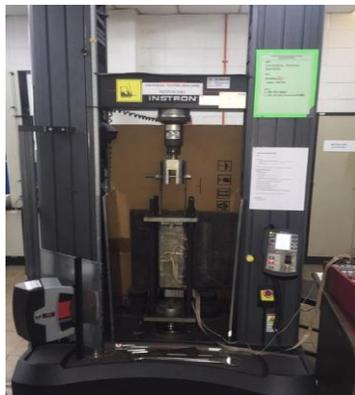
Figure 14: Instron 5982 Universal Testing Machine
