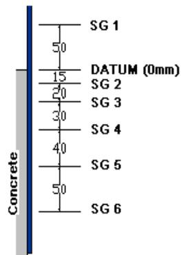
Figure 12: Strain gauges locations along bond length
