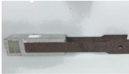
Figures8: SPECS-7 with corroded steel plate
