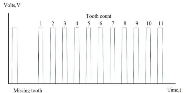
Figure 10. An example of the 12-1 trigger wheel signal
