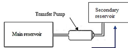
Figure 5. Fuel transfer concept of the test bench.
