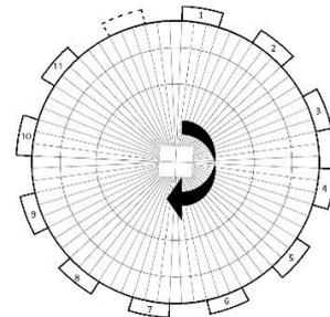
Figure 9. 12-1 trigger wheel
