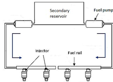
Figure 4. Fuel system concept of the test bench.
