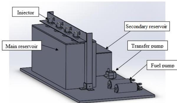
Figure 3. Design of the test bench
