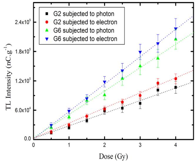
Fig. 3. Dose response of G2 and G6 subjected to photon and electron from LINAC irradiation at 6 MV and 6 MeV.
