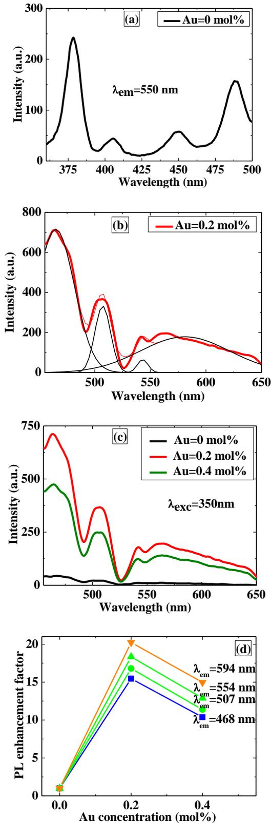
**Figure 4** (a) Excitation spectrum of the glass samples in range of 360 to 500 nm; (b) PL spectra for glass containing 0.2 mol% Au with Gaussian fit; (c) Luminescence spectra for all samples under 350 nm excitations; (d) PL enhancement factor showing enhancement and quenching ratio for respective glass samples with varying Au concentration
