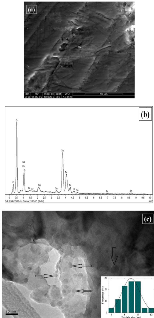
**Figure 3** (a) FESEM image at specific region of glass sample containing 0.4 mol% Au; (b) the respective EDX spectra of glass sample; (c) TEM image of the Au NPs (glass containing 0.4 mol% Au) show closely dispersed particles, majority with non-spherical shape. Inset shows histogram of Au NPs with average diameter of  $\approx 9$  nm
