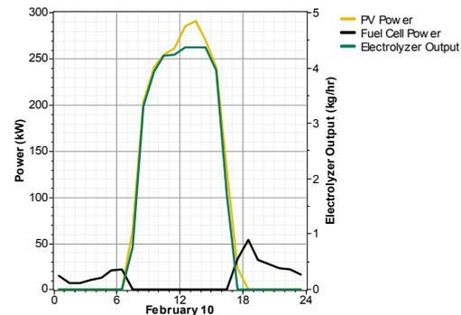
Figure 18. Contribution of electric energy production by various energy sources in an optimal system
