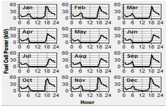
Figure 9. Daily profile of fuel cell out
