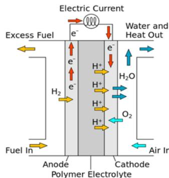
Figure 6. The basic principle of a fuel cell
