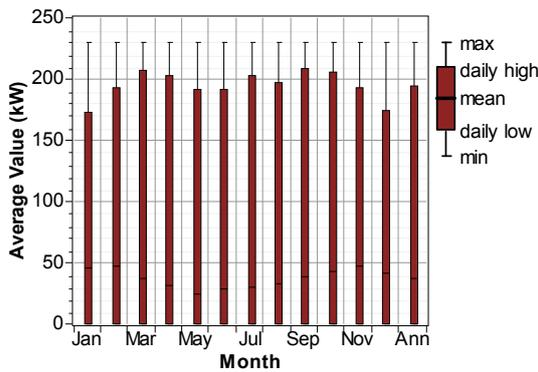
Figure 12. Monthly average electricity consumed by the electrolyzer
