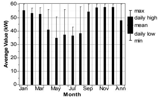
Figure 10. Monthly average output of fuel cell
