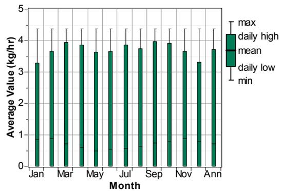
Figure 13. Monthly average output of the electrolyzer
