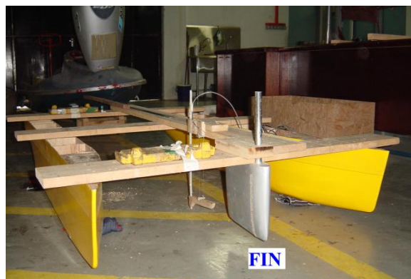
Figure 2b Fin attached to the catamaran hull at centerline
