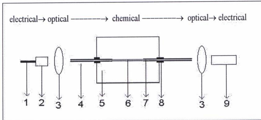
**Figure 1.1:** The command transduction steps of a chemical optical fiber chemical sensor. In this case (1) is current supply (2) light source (3) optical lens (4) optical fiber cladding (5) test sample (6) sensing element of the fiber (7) fiber core (8) connection protector (9) optical power detector.
