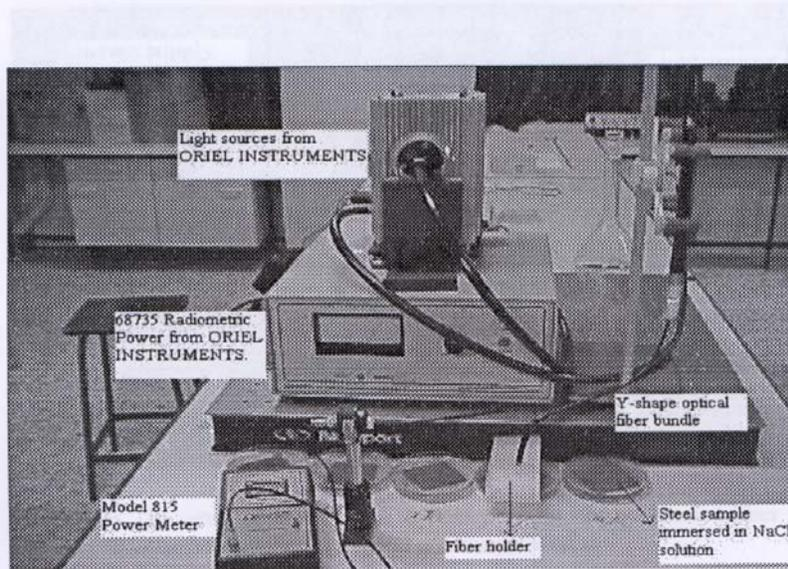
Photo 1.1: Set-up of the Fiber Optic bundle for steel corrosion when immersed in NaCl solution.
