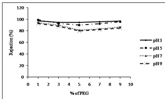
Figure 3 Rejection (%) of BSA using PSf-based membrane
