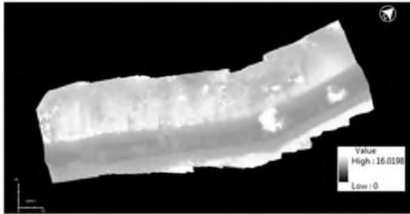
**Figure 5.** DTM extracted from Y6 UAV imagery (40m altitude).
