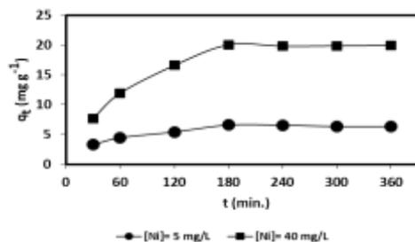
**Figure 2** Kinetic data for Ni(II) uptake by Fe<sub>3</sub>O<sub>4</sub> MNPs. Conditions: weight of adsorbent 60.0 mg, Ni(II) concentration = 5.0 and 40.0 mg L<sup>-1</sup>, volume of solution = 100 mL, pH 6.0, Temperature = 25°C, contact time from 30 - 360 min.
