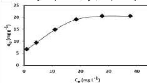
**Figure 1** Adsorption capacity of Ni(II) on Fe<sub>3</sub>O<sub>4</sub> MNPs. Conditions: weight of adsorbent 60.0 mg, Ni(II) concentration ranged from 5.0 - 50.0 mg L<sup>-1</sup>, volume of solution 100 mL, pH 6.0, Temperature = 25°C, contact time = 180 min
