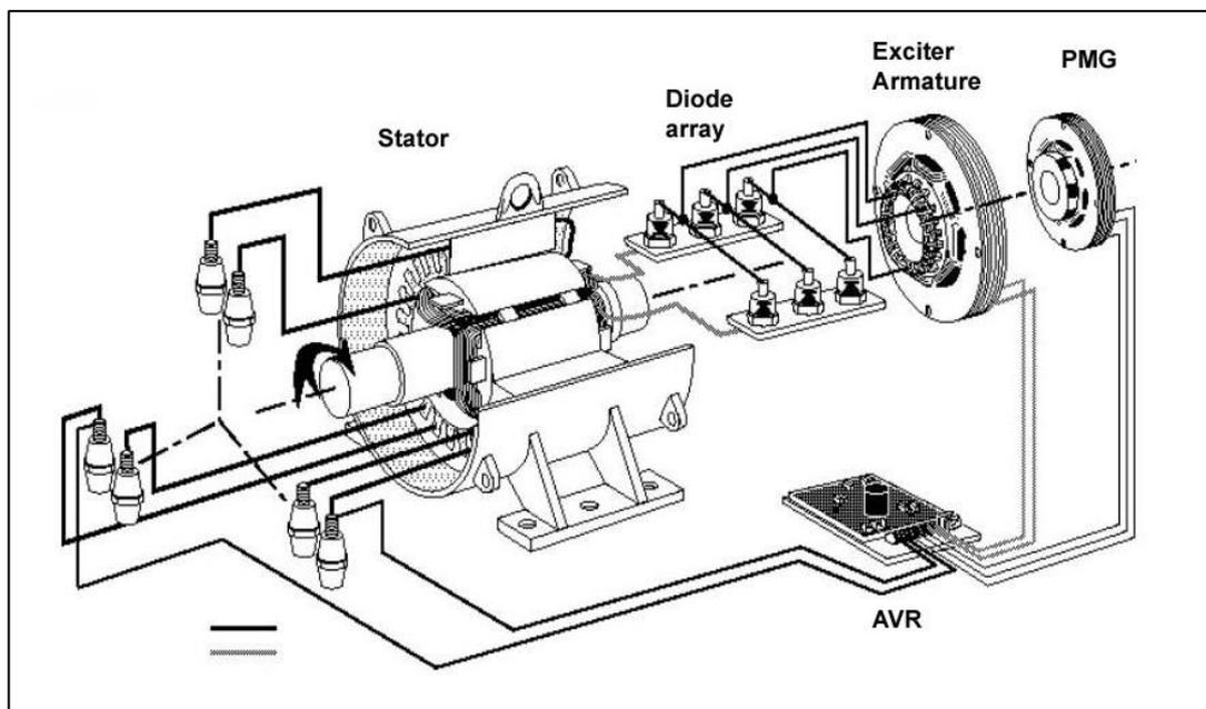
Figure 1.2: AVR system for Power Generator
