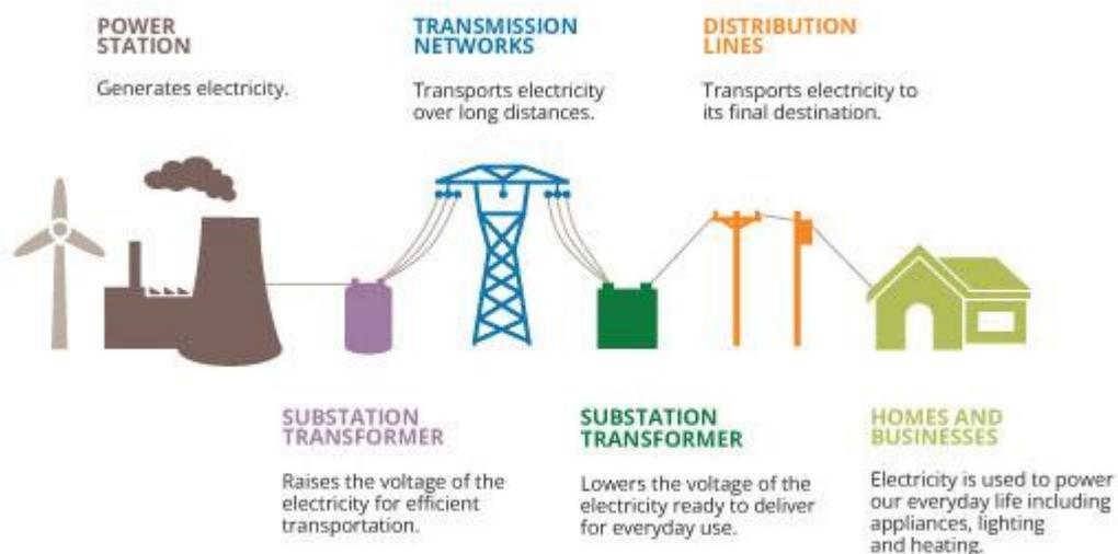
Figure 1.1: Typical Power System Network
