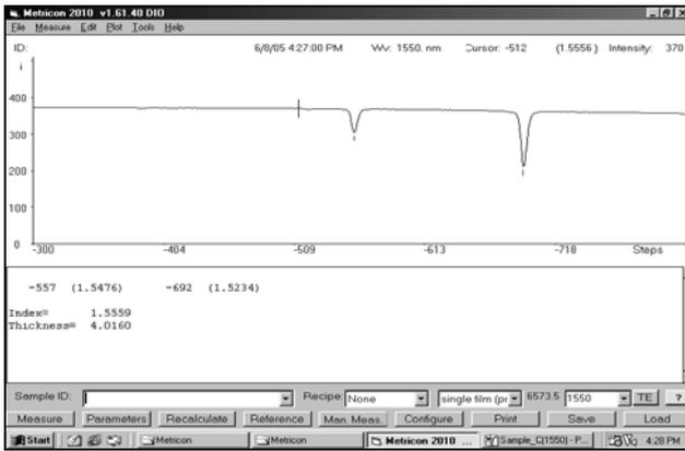
Figure 3. Graphical output from prism coupling measurement
