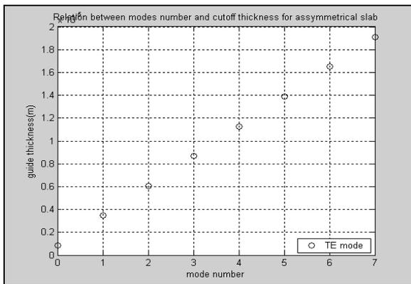
Figure 8. Film cutoff thickness for confined modes
