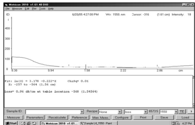
Figure 7. Fiber detected power against slab distance
