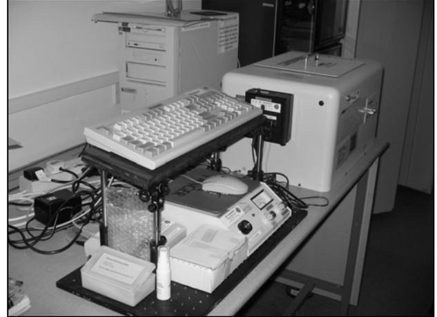
Figure 2. Metricon™ prism coupler
