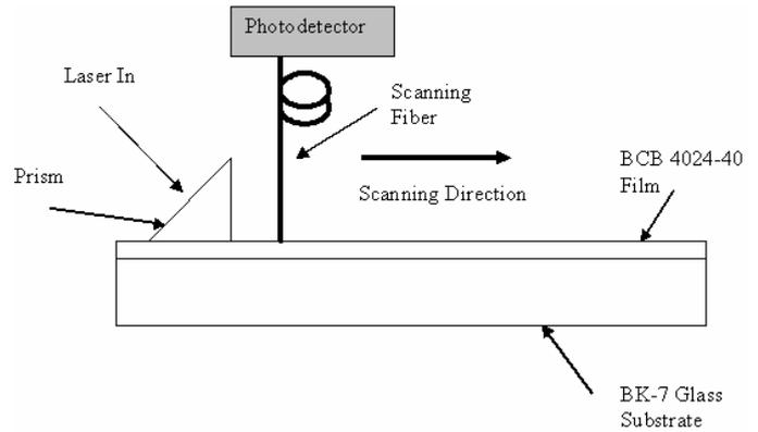
Figure 6. Prism coupling measurement setup of slab loss
