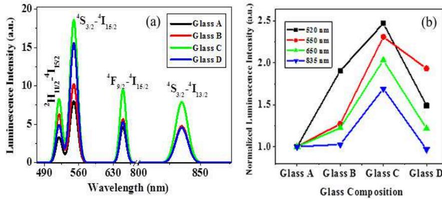
**Fig. 3:** (a) Luminescence spectra of glasses under an excitation of 786 nm i) Without AgCl (A), with ii) 0.1 mol% (B), iii) 0.5 mol% (C), iv) 1.0 mol% (D) AgCl (b) plot of emission intensity versus concentration of Ag (mol%). Maximum amplification for the green and red bands occurred for 0.5 mol% Ag.
