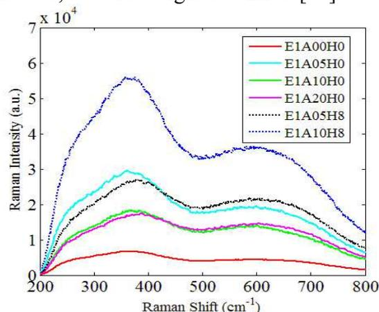
**Fig. 2:** Raman signals of the samples  $\text{ExAyHz}$ , where  $x=1$  mol% is the concentration of erbium ions,  $y=0, 0.5, 1$  and  $2$  mol% is the concentration of the AgCl, and  $z=0$  and  $8$  is the annealing time for the zinc-tellurite glass.
