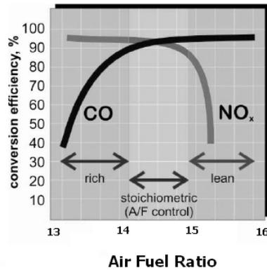
Figure 1: Relationship between conversion efficiency and air fuel ratio.
