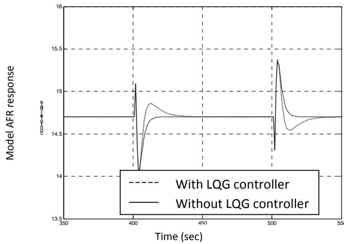
Figure 9. AFR response with LQG controller (dashed) and without LQG controller (solid).
