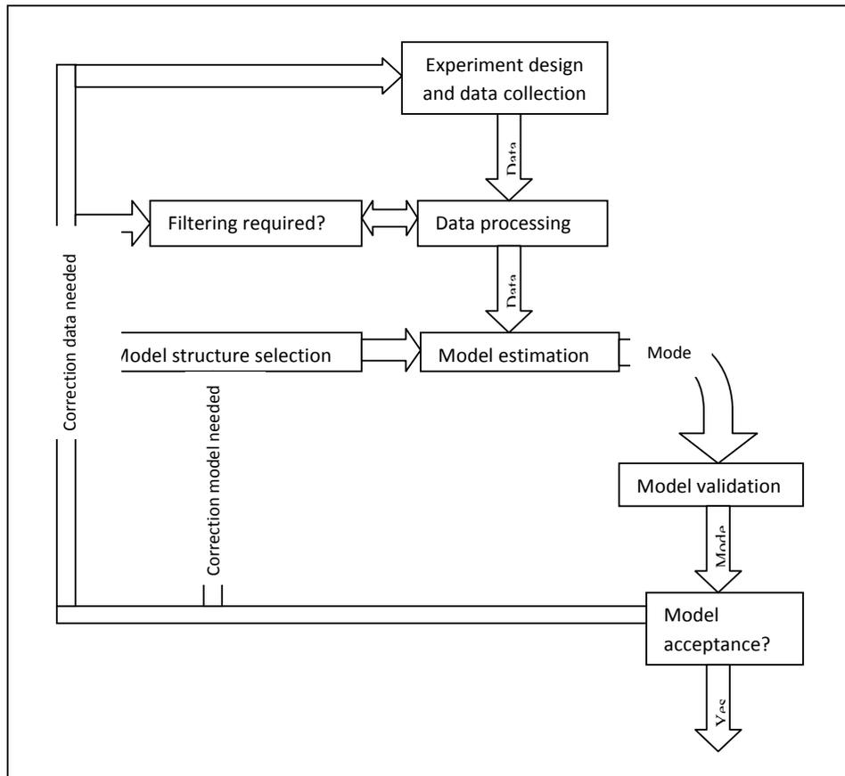
Figure 3: Cycle of system identification function.
