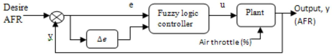
Figure 7. The Fuzzy Logic controller and engine model in MATLAB-SIMULINK.
