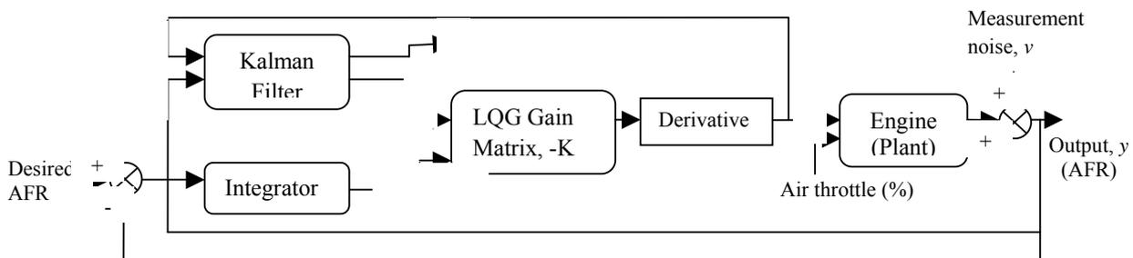
Figure 5. Block diagram engine system controlled by the LQG controller.
