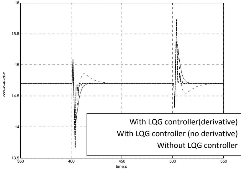
Figure 10. AFR response with LQG controller (with and without the derivative block).
