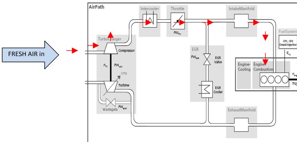
Figure 2: Schematic of air system.
