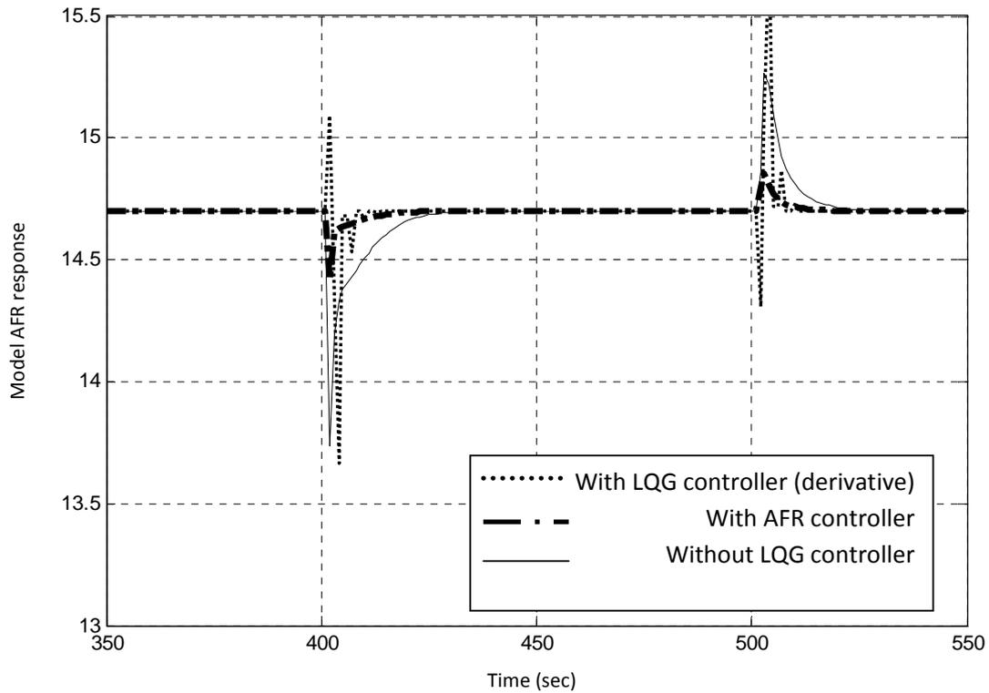
Figure 11. AFR response from engine model with fuzzy logic controller and LQG controller crop from time between 350s to 550s.
