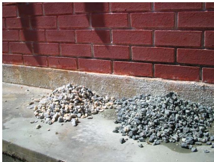
Figure 1.2: Sample of aggregates (left is limestone, right is granite).
