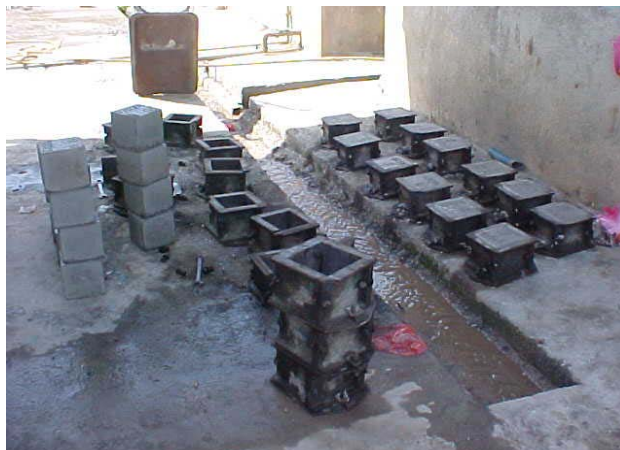
Figure 1.3: Sample of concrete cube with 150 x 150 x150 in size.
