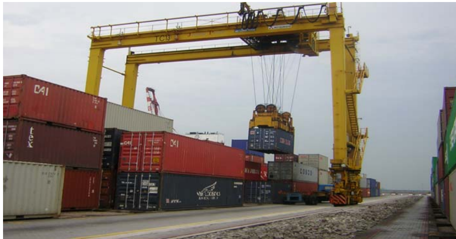
Figure 1-4 Yard crane Operations off-loading container from truck for stacking at yard
