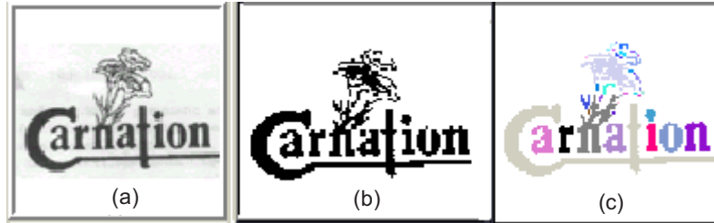
Figure 4 Component labeling: (a) A logo containing connected components, (b) Result of automatic thresholding, (c) Result of component labeling
