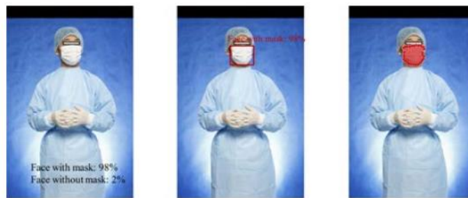
Figure 1.5 Three tasks of computer vision on face mask detection example, classification (left), object detection (middle) and segmentation (right) [2]
