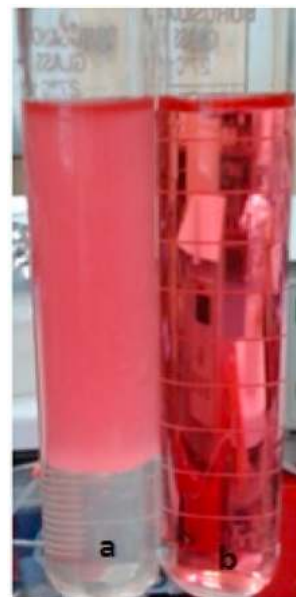
Fig. 27. Cloudy (a) vs clear oil (b) produced during tertiary and secondary flooding, respectively.
