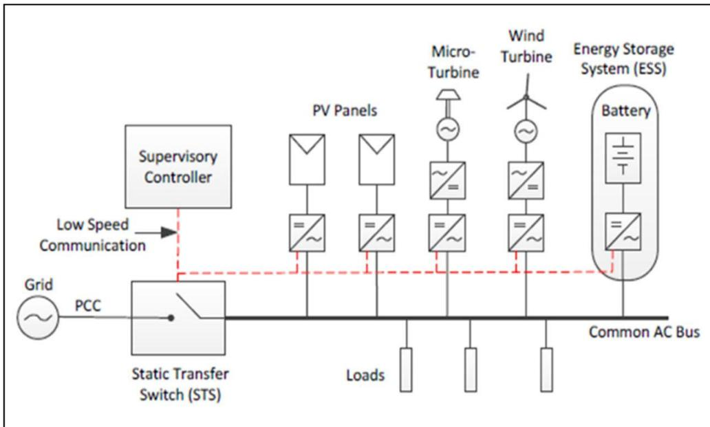
Figure 1.1 Typical configuration of integrated distributed generator
