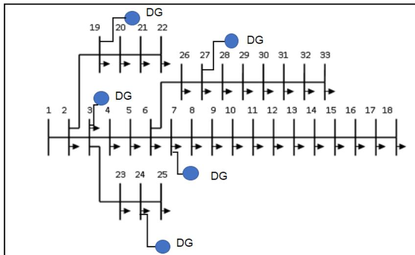
Figure 1.5 IEEE 33 bus system with distribution generators connected.
