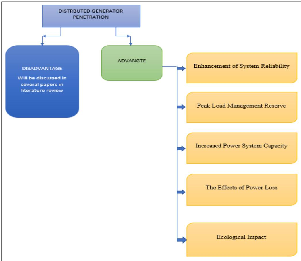
Figure 1.2 Distributed Integrated Generation's Advantages
