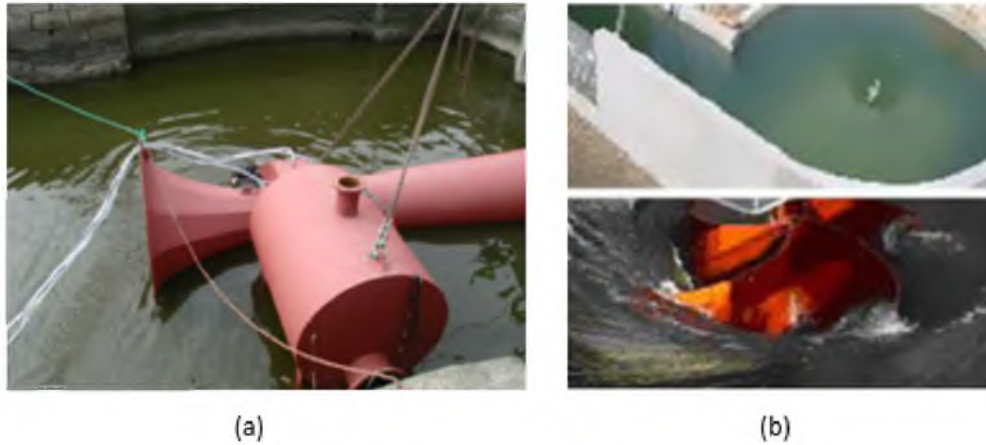
Figure 1.1 Examples of turbine systems (a) HydroVenturi TM; (b) (GWVPP) TM. (Khan et al. , 2009a)
