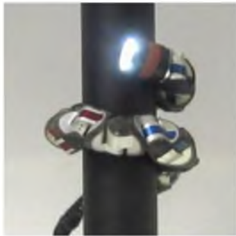
c) Unified snake robot for pipe inspection which is developed by Howie Choset group at CMU's Biorobotics Lab (Rollinson, Buchan and Choset, 2012)
