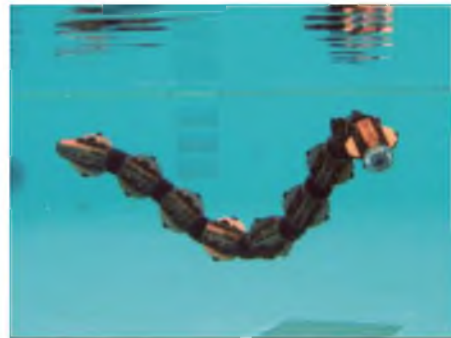
d) An amphibious snake-like ACM-R5 robot developed by Prof. Hirose (Hirose and Yamada, 2009)
