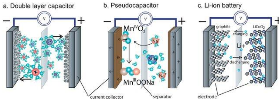
Figure 1.1 Schematic drawing of (a) EDLC (b) pseudocapacitance type of supercapacitors and (d) Li-ion battery (Jost et al., 2014).
