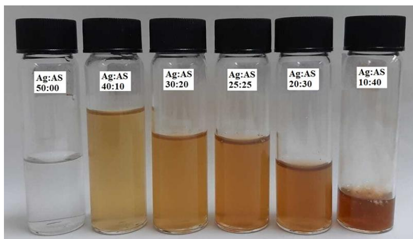
Figure 2. The colour changes on the solutions at different silver nitrate: acetylated starch ratio.
