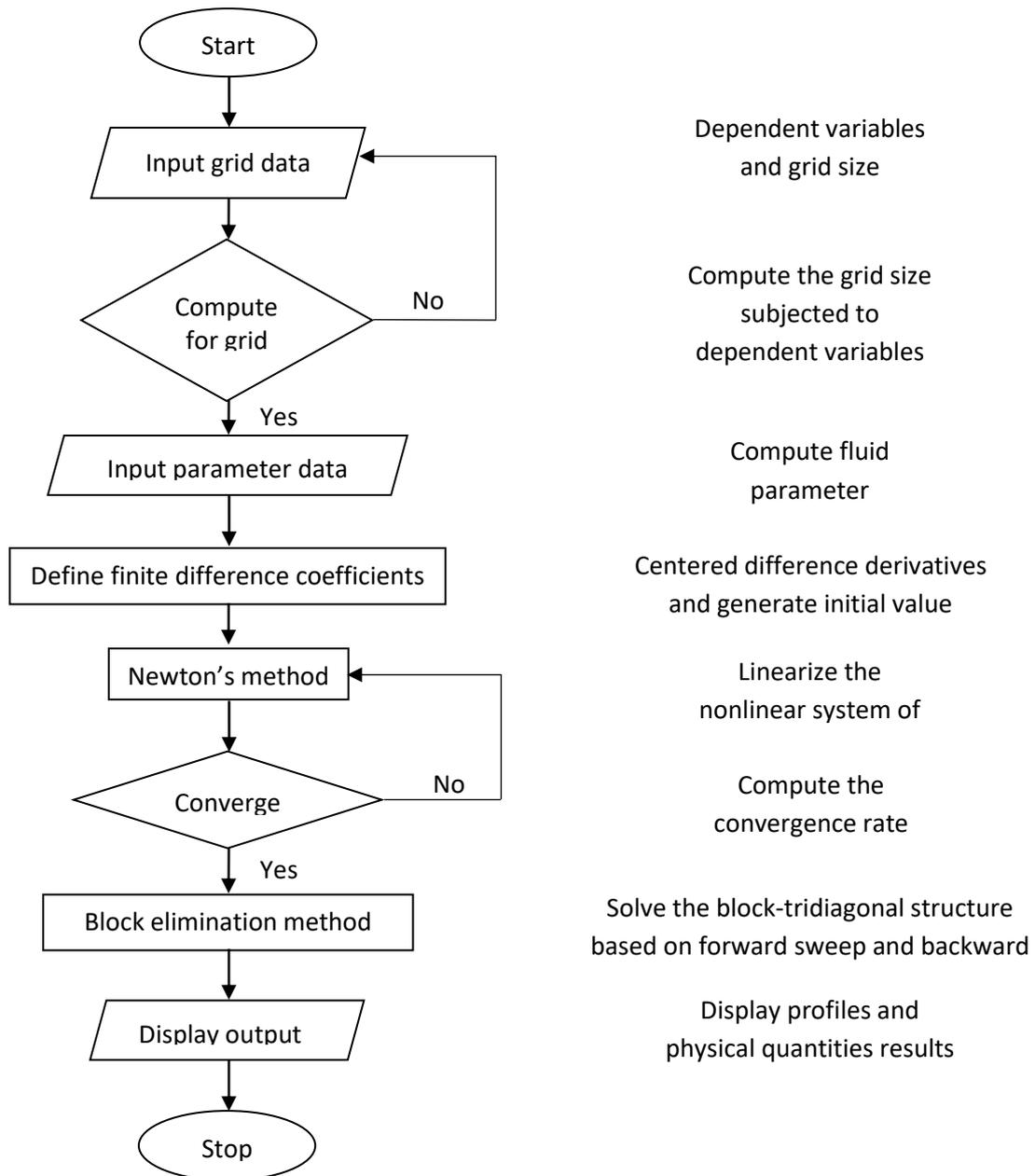
Fig. 2. Flow diagram for the Keller box method
