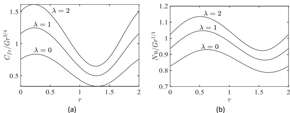
**Fig. 5.** The physical quantities in (a) skin friction coefficient and (b) Nusselt number of various values of the nonlinear thermal parameter  $\lambda$  with fixed parameter  $c = 0.5, \Omega = 0.2, \phi = 0.05, Pr = 6.2, \varepsilon = 0.5$
