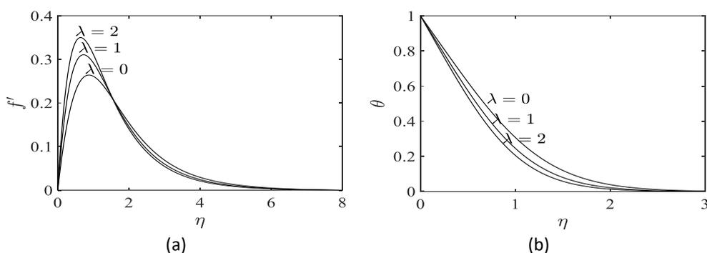
**Fig. 4.** The behavior of (a) velocity profile and (b) temperature profile due to various values of the nonlinear thermal parameter  $\lambda$  with fixed parameter  $c = 0.5, \Omega = 0.2, \phi = 0.05, Pr = 6.2, \varepsilon = 0.5$
