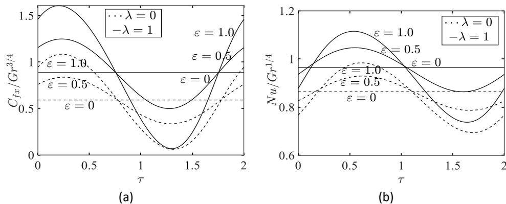
**Fig. 6.** The physical quantities in (a) skin friction coefficient and (b) Nusselt number various values of the amplitude of modulation  $\varepsilon$  with fixed parameter  $c = 0.5$ ,  $\Omega = 0.2$ ,  $\varepsilon = 0.5$ ,  $Pr = 6.2$
