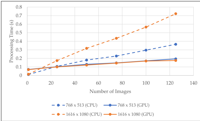
Figure 7: The CPU and GPU processing time for different number of image and image pixels for kernel 3.
