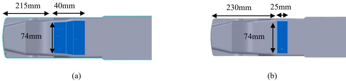
Fig. 2 - Two different locations of the frontal deflector to be mounted (a) location for FD 1, FD 2 and FD 3; (b) location for FD 4, FD 5 and FD 6
