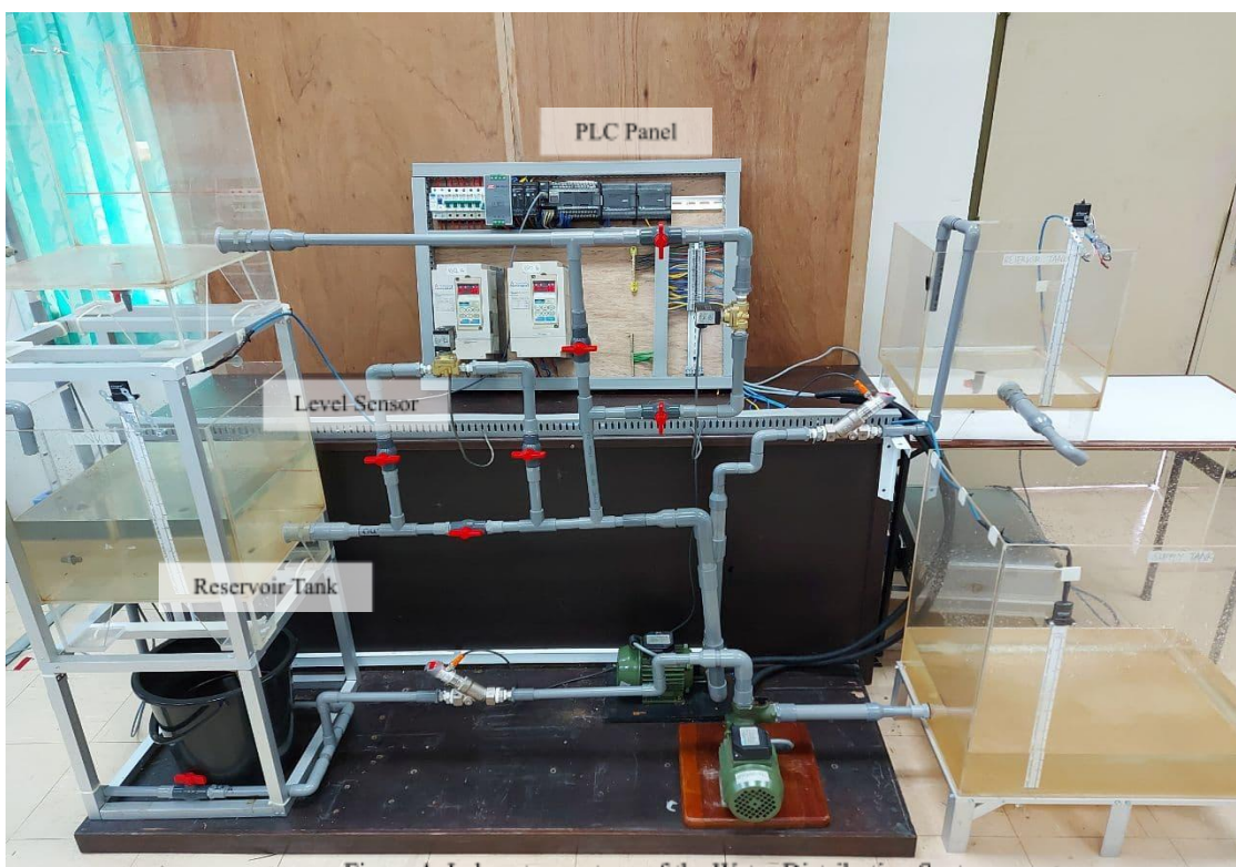
Figure 1. Laboratory set-up of the Water Distribution System
