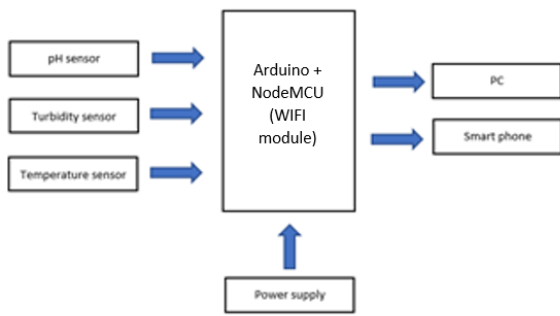
Figure 6. Block Diagram of the project
