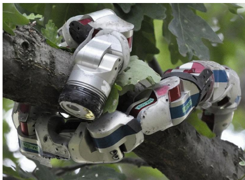
Figure 1.1 Snake-like robot with rigid structure [1]
