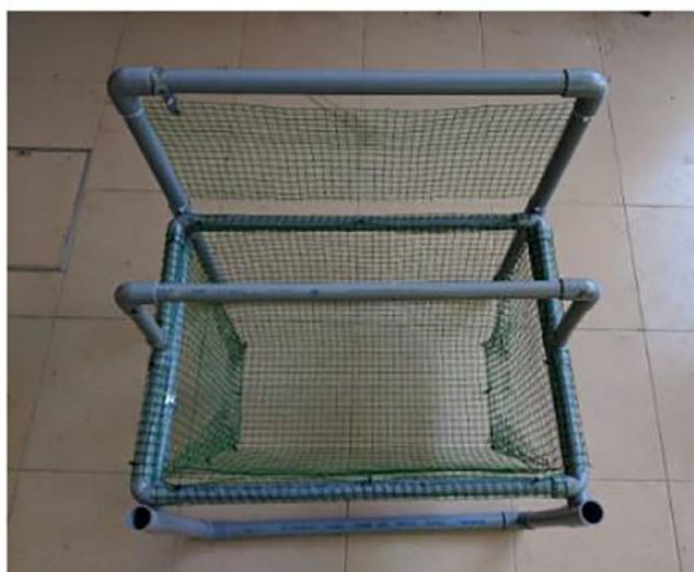
Fig. 7. Trash trap to collect diverted trashes.
