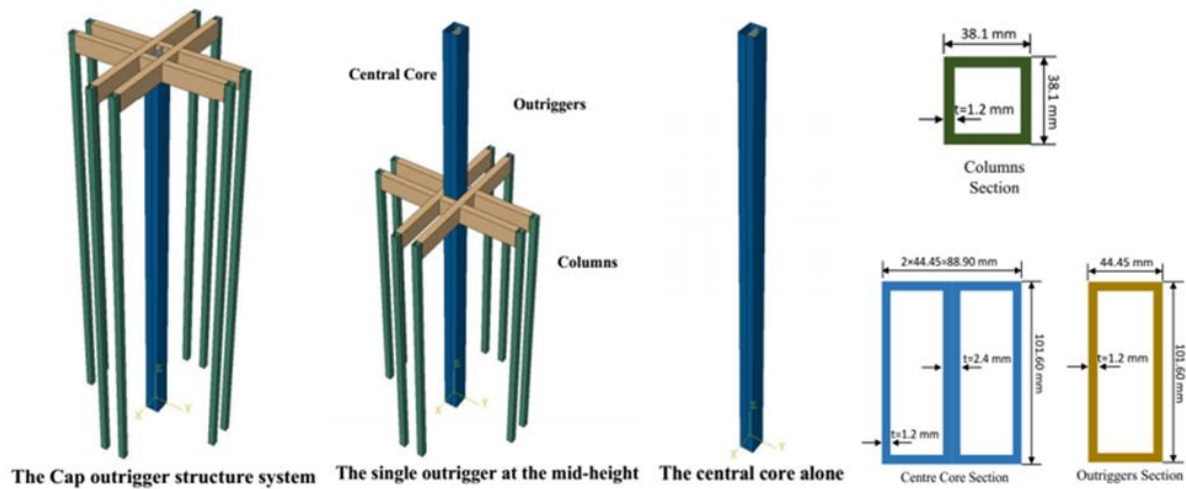
Figure 4. Cap outrigger structure, optimal outrigger structure, the central core alone, section size of the components.
