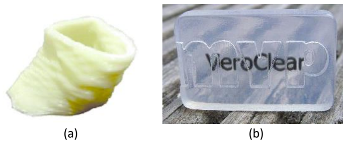
Fig. 1. Example of model created using (a) ABS plastic material and (b) VeroClear resin
