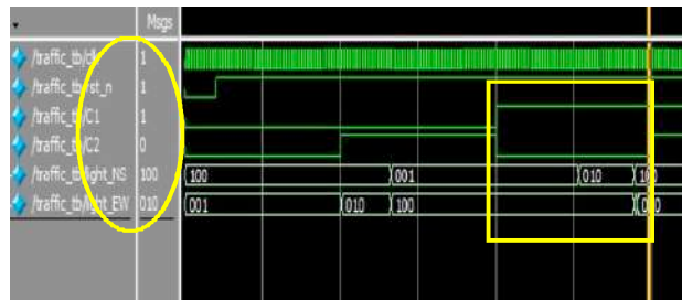
Figure 6: Simulation waveform when sensor C1 is active('1') and C2 not active('0')
