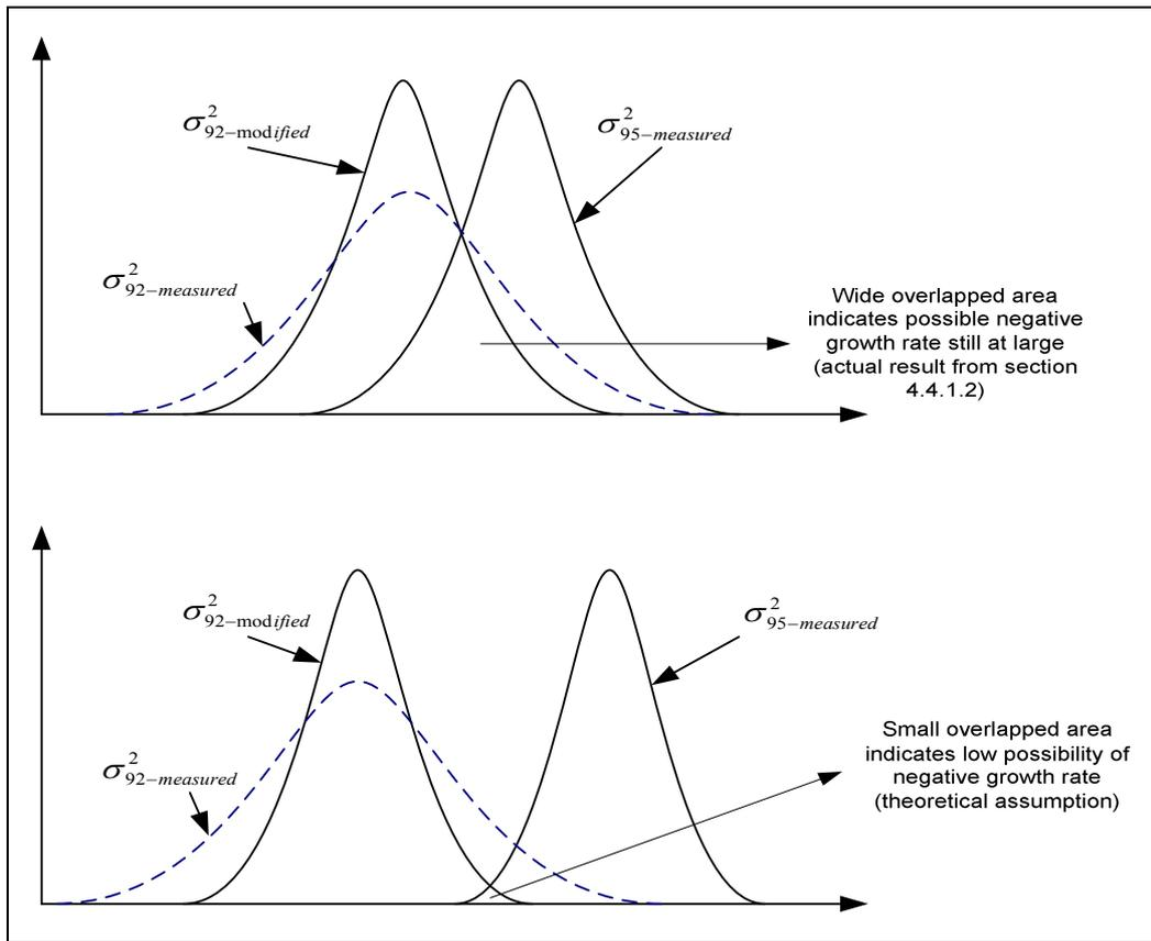
Figure 3.15b: Illustration of modified corrosion rate.
