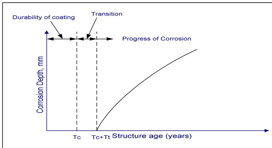
**Figure 3.17: The corrosion initiation time of coated structures [Paik and Thayambali, 2002]**
