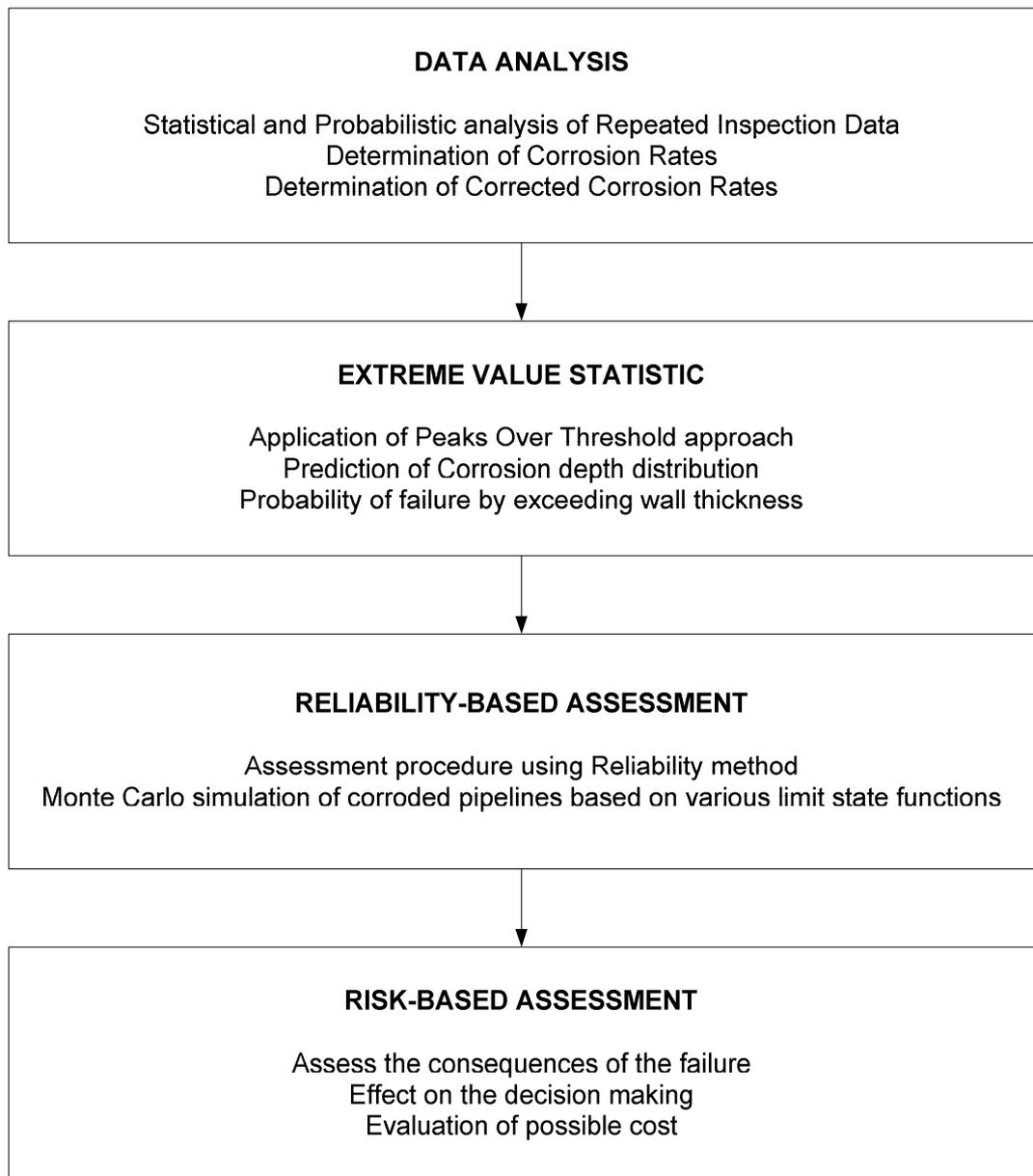
**Figure 2.3: A general summary of overall procedure on the use of inspection data in the structural reliability assessment of corroding pipelines as proposed by Yahaya [1999].**
