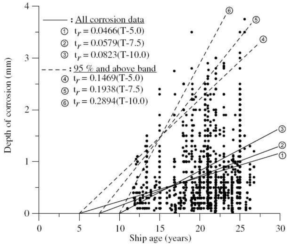
**Figure 4.3 Comparison of annualized corrosion rate formulations, together with the measured corrosion data for seawater ballast tanks [Paik and Thayambali, 2001].**
