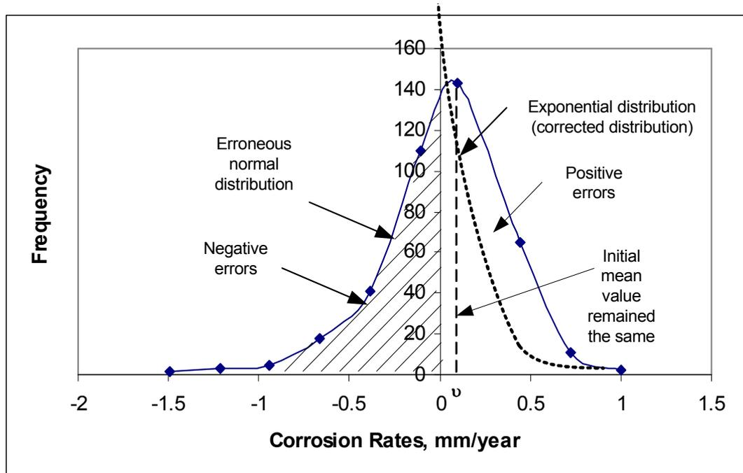
Figure 3.16: Exponential distribution extracted from Normal distribution of actual corrosion rate,  $CR_{A90-92}$ , with mean value given by sample mean from normally distributed raw data.
