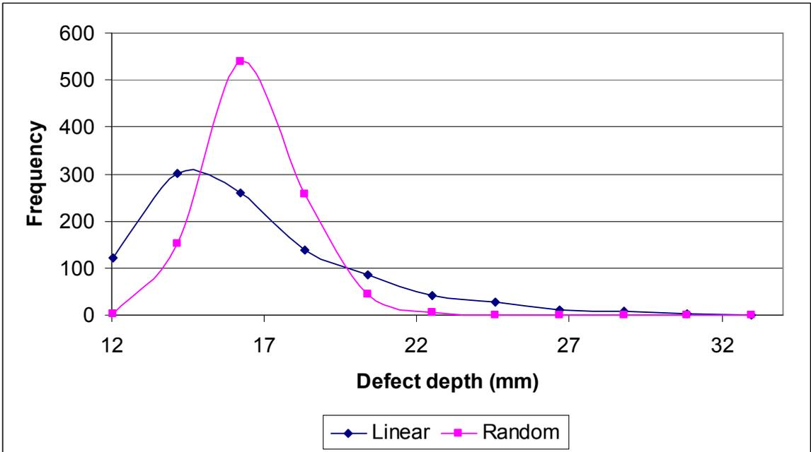
**Figure 3.33: Comparison of predicted extreme corrosion depth to actual depth in year 2010 using linear and random models (*Pipeline B*)**
