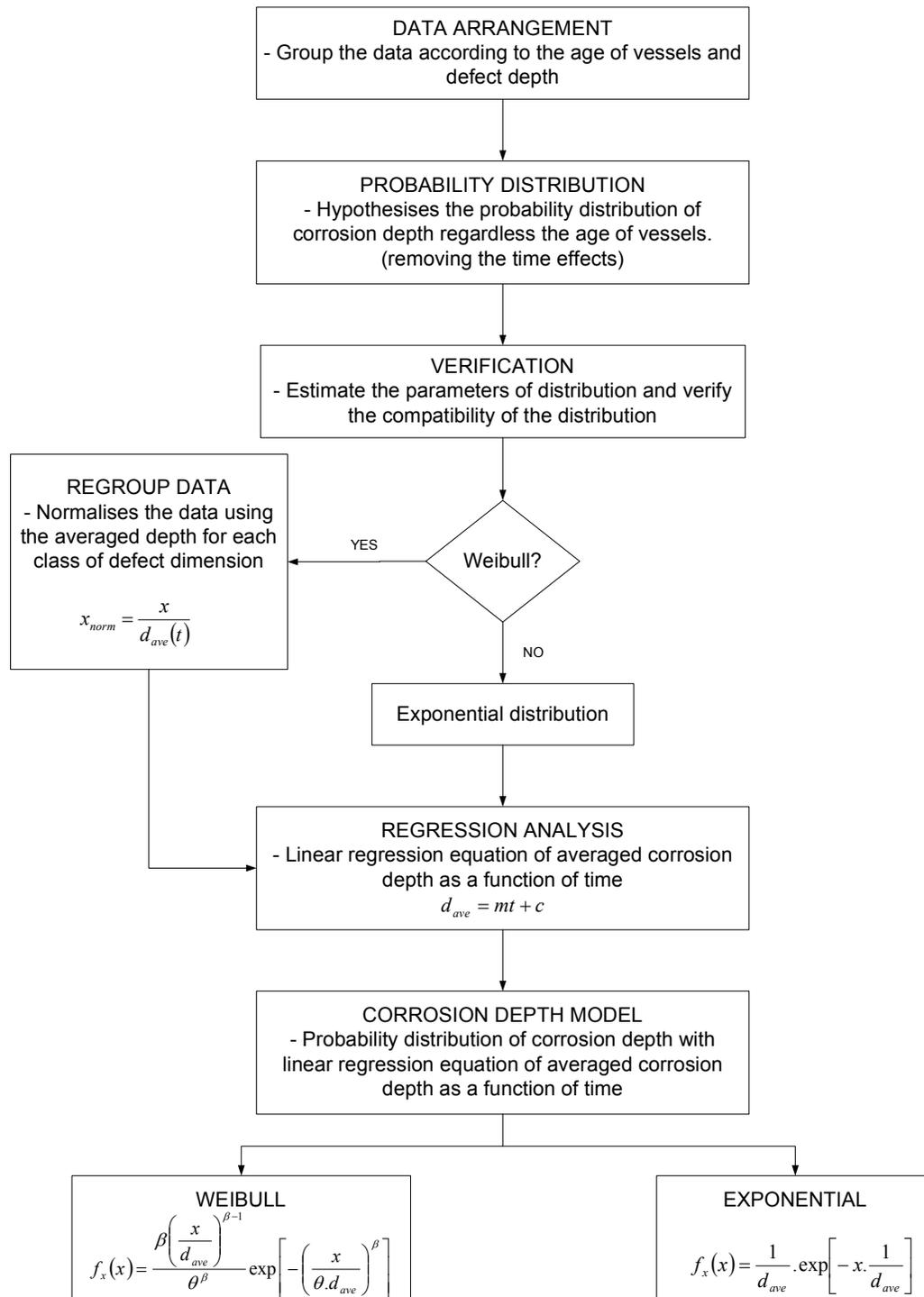
**Figure 4.20: Flow chart of a development of corrosion depth distribution with defect depth as a function of time.**
