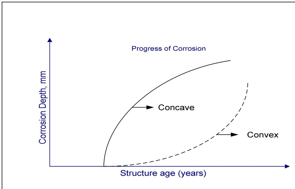
**Figure 2.2: Corrosion progress model**
