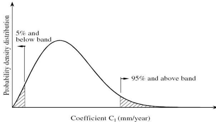
**Figure 4.2: The 95 percentile and above band for developing the severe (upper bound) corrosion wastage model [Paik and Thayambali, 2001].**
