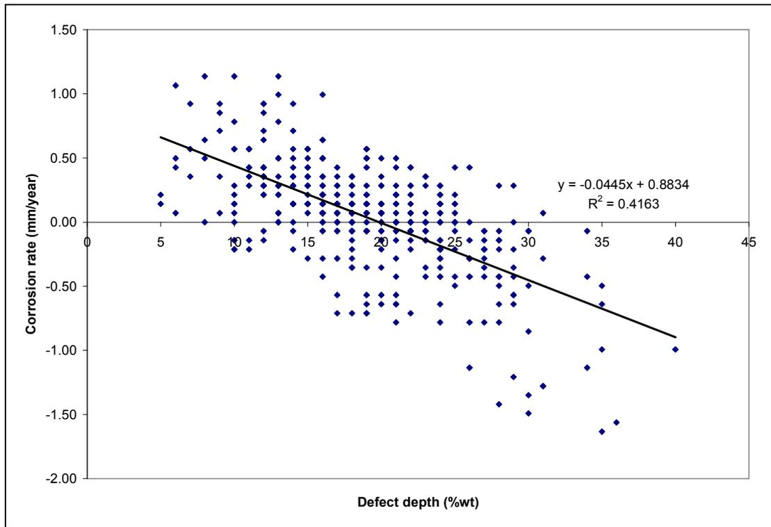
**Figure 3.6: Corrosion rate,  $CR_{A90-92}$  plotted against defect depth  $d_{A92}$  with linear regression line.**
