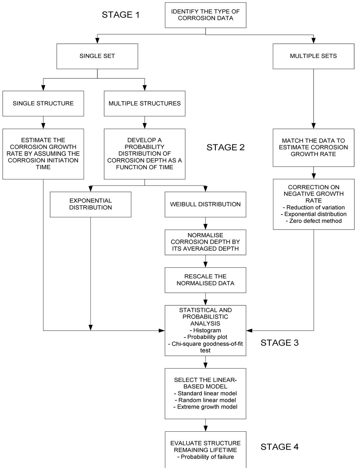
**Figure 5.2: Detail illustration of the component of generic assessment procedure for corrosion data and structure reliability analysis.**
