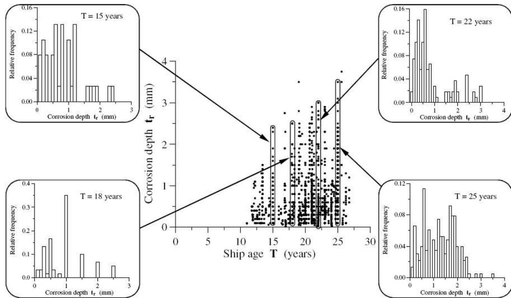
**Figure 4.1: The corrosion depth versus the ship age from thickness measurements of seawater ballast tank structures [Paik and Thayambali, 2001].**
