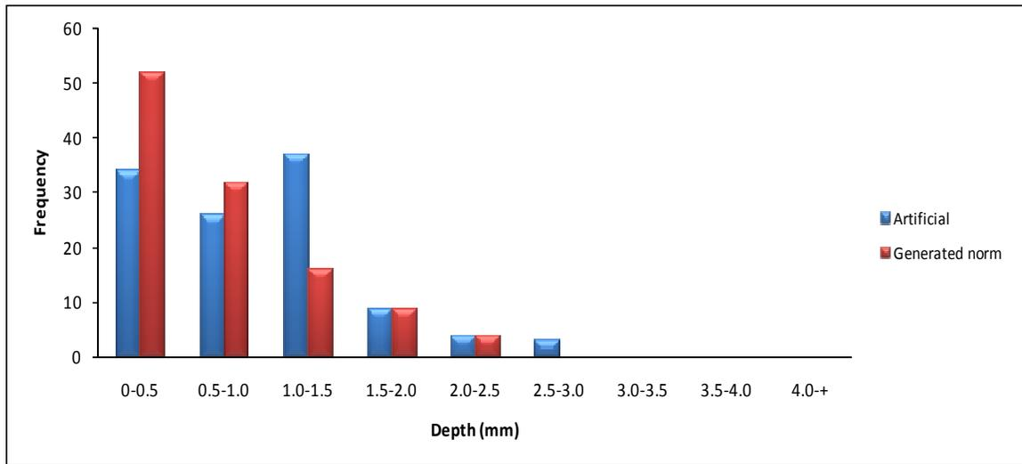
Figure 4.13: Comparison of predicted depth data to actual data for vessel age of 18-18.5 years old (RMSE of  $\pm 11.62$ )
