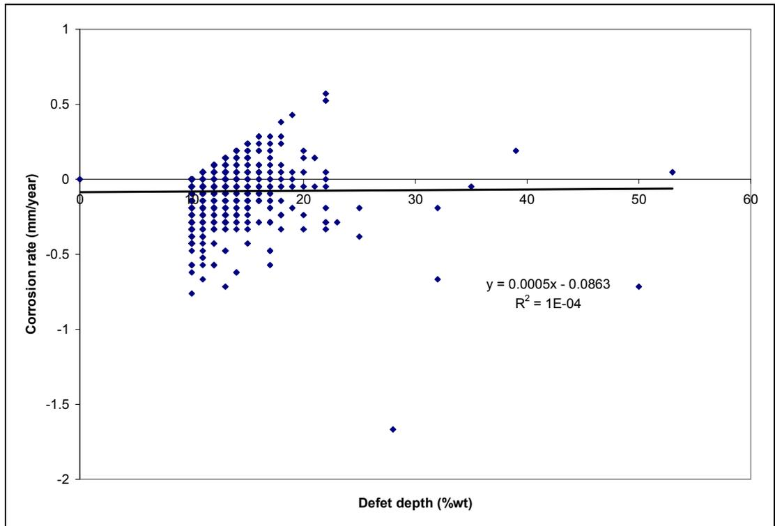
Figure 3.5: Corrosion rate,  $CR_{C98-2000}$  plotted against defect depth,  $d_{C-2000}$  with linear regression line.
