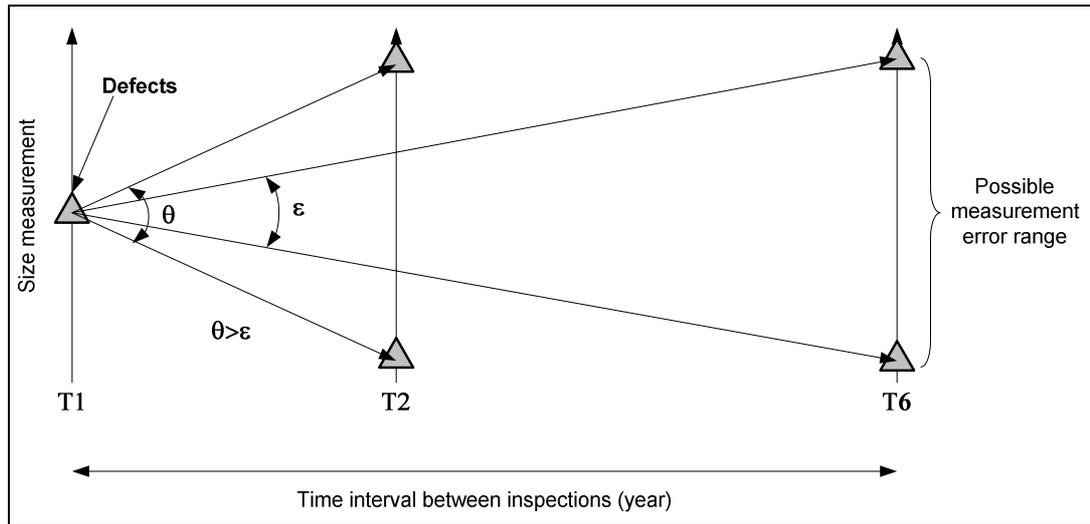
**Figure 3.8: Illustration of the Time interval-based error theory. The uncertainty produced by measurement error upon growth rate reduces as the interval increases.**
