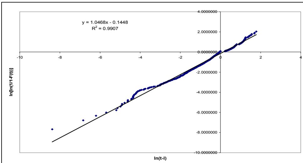
Figure 4.11: Weibull probability plot of rescaled data
