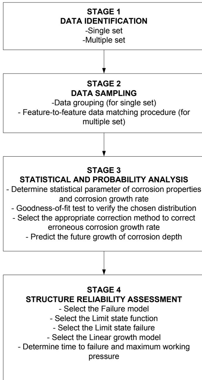
**Figure 5.1: General illustration of the proposed assessment procedure for corrosion data and structure reliability analysis.**
