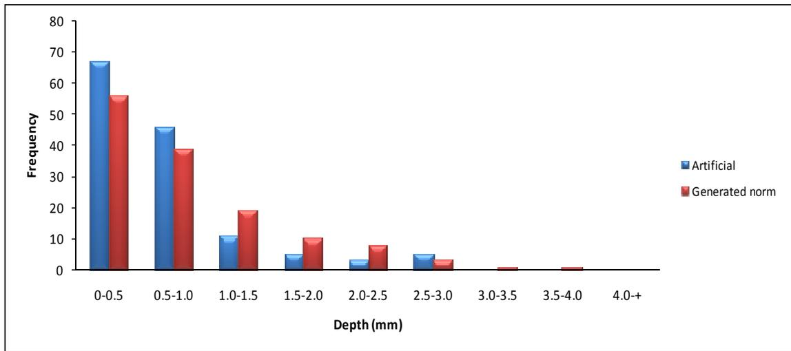
Figure 4.16: Comparison of predicted depth data to actual data for vessel age of 23-23.5 years old
