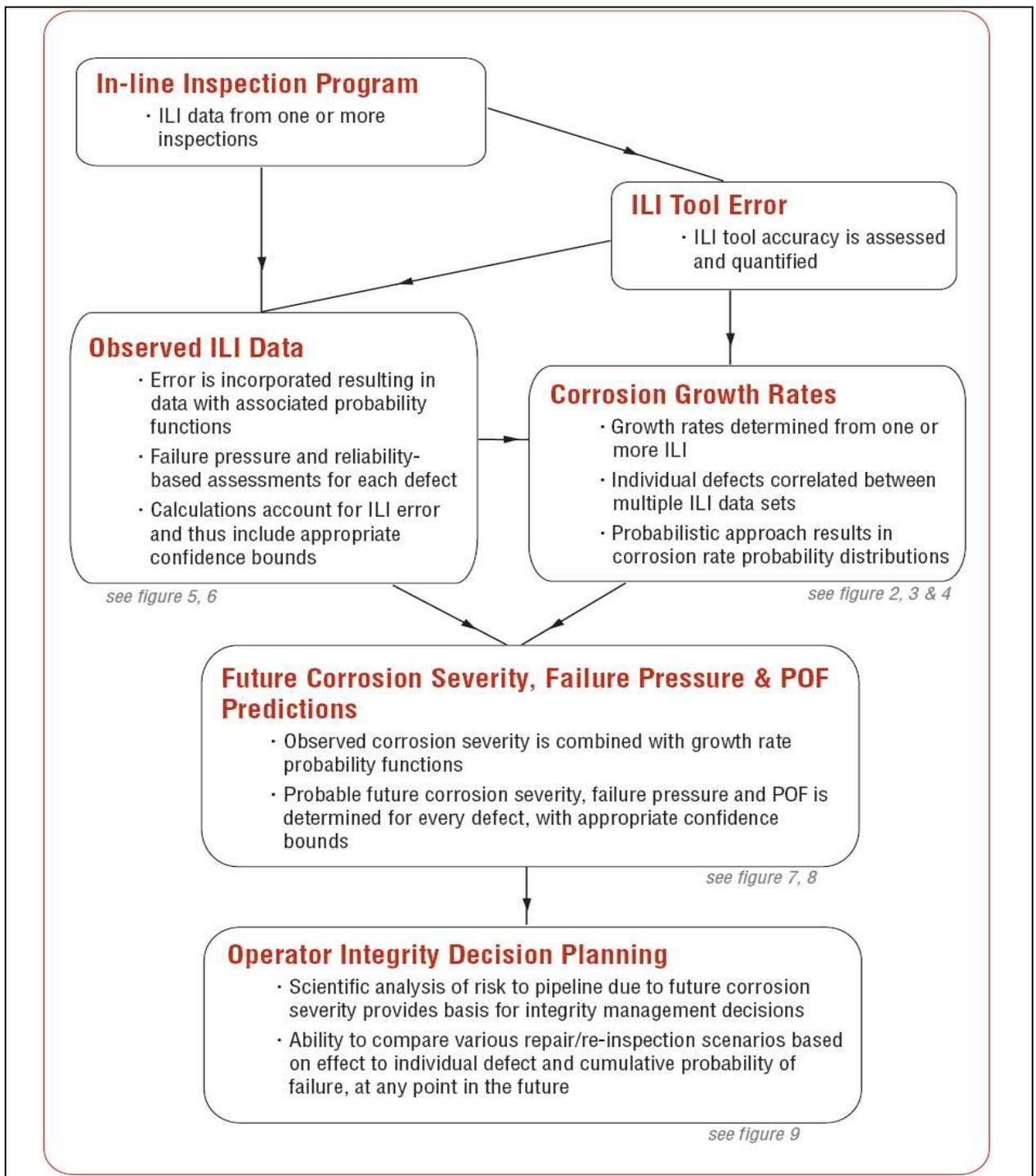
**Figure 2.4: Corrosion growth analysis and probability of failure methodology by Desjardins [2002a and 2002b].**
