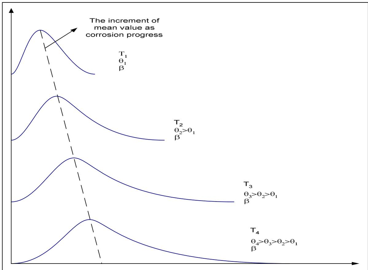
**Figure 4.8: The increment of the Weibull scale parameter as corrosion progress for normalised data.**
