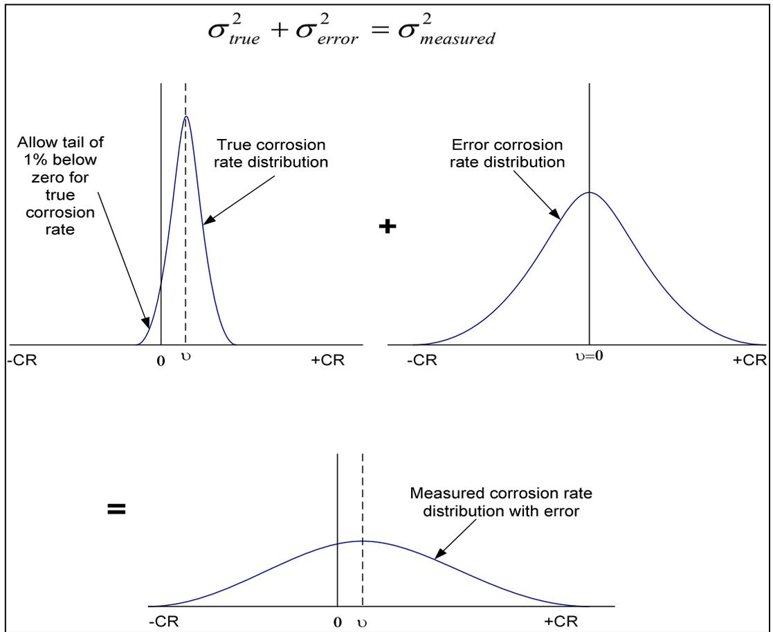
**Figure 3.13: The relationships between measured, ‘true’ and error corrosion rates distribution according to Yahaya [1999].**
