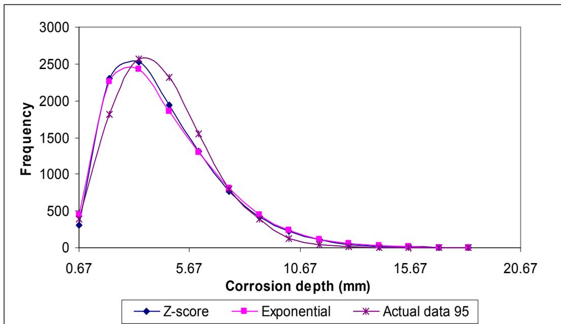
**Figure 3.19: Comparison result: Prediction of data from 1992 to 1995 using corrected corrosion growth rate (*Pipeline B*).**
