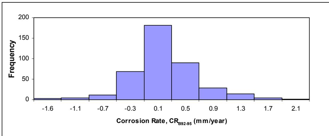
Figure 3.11: The histogram of corrosion rate,  $CR_{B92-95}$  (*Pipeline B*)
