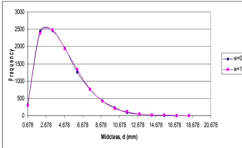
**Figure 3.24: Comparison of predicted defect depth to actual depth based on extreme growth model and partial factor of 0 and 1 (*Pipeline B*)**
