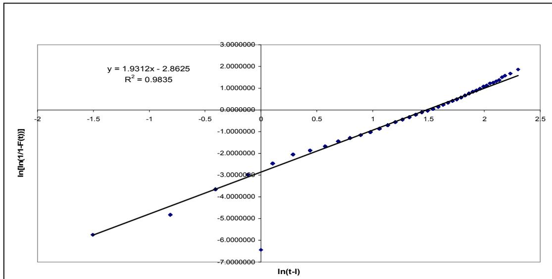
Figure 3.12: The Weibull Probability plot for corrosion depth,  $d_{B95}$  (*Pipeline B*)
