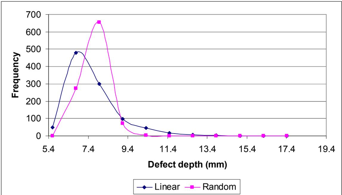
**Figure 3.31: Comparison of predicted extreme corrosion depth to actual depth in year 2010 using linear and random models (*Pipeline A*)**
