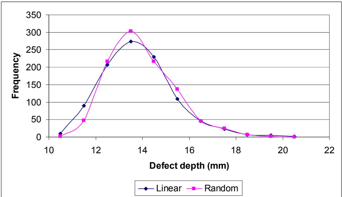
**Figure 3.32: Comparison of predicted corrosion depth to actual depth in year 1995 using linear and random models (*Pipeline B*)**
