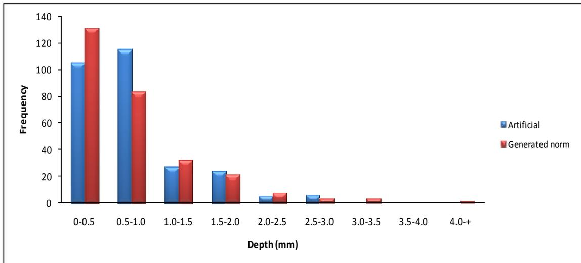
Figure 4.14: Comparison of predicted depth data to actual data for vessel age of 21-21.5 years old (RMSE of  $\pm 14.84$ )
