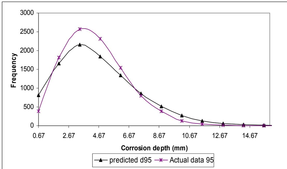
**Figure 3.18: Comparison result: Prediction of data from 1990 to 1995 using uncorrected corrosion growth rate (*Pipeline A*).**
