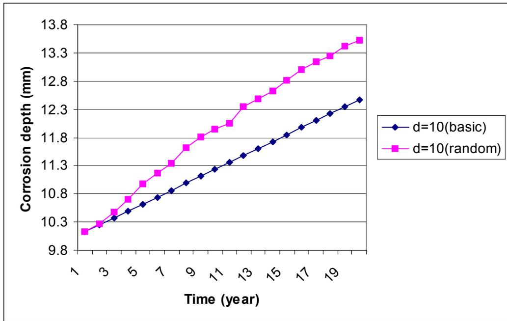
**Figure 3.28: Linear prediction of corrosion defects by using basic and random linear models (d=10mm)**
