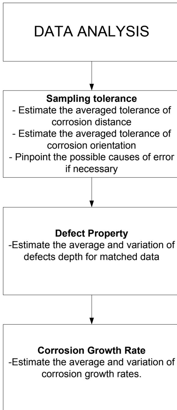
**Figure 3.3: The flow chart of statistical analysis on matched defects**
