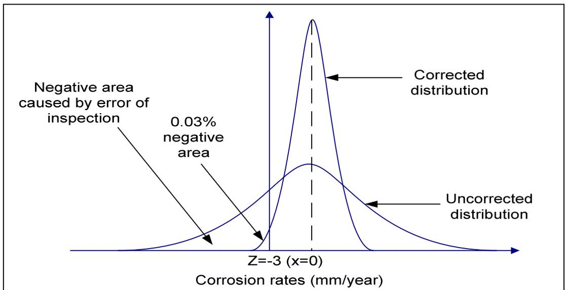
**Figure 3.14: Corrected corrosion rates distribution ( $CR_{B92-95}$ ) using Z-score correction method.**
