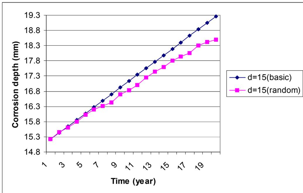
**Figure 3.29: Linear prediction of corrosion defects by using basic and random linear models (d=15mm)**
