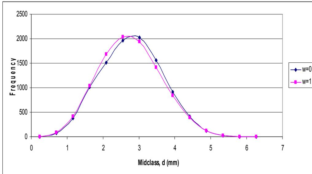
**Figure 3.22: Comparison of predicted defect depth to actual depth based on extreme growth model and partial factor of 0 and 1 (Pipeline A)**
