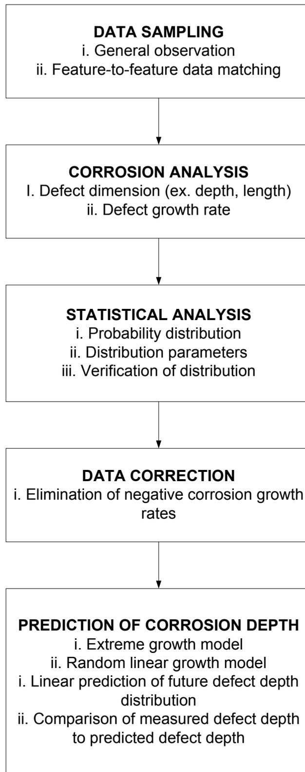
**Figure 3.34: The proposed methodology of corrosion defect analysis of pipelines**
