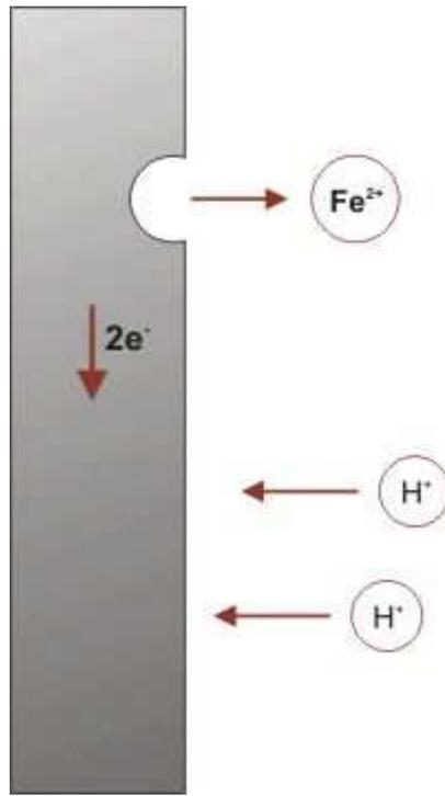
**Figure 2.1: Corrosion Electrochemical Process**
