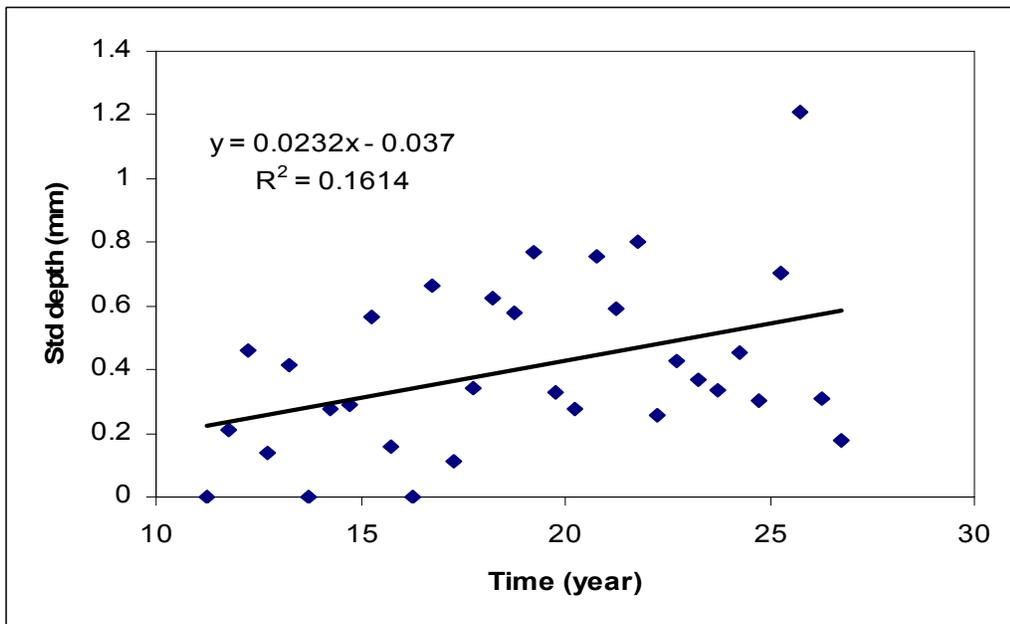
Figure 4.5: Linear regression analysis of *standard deviation* of defect depth and vessel age
