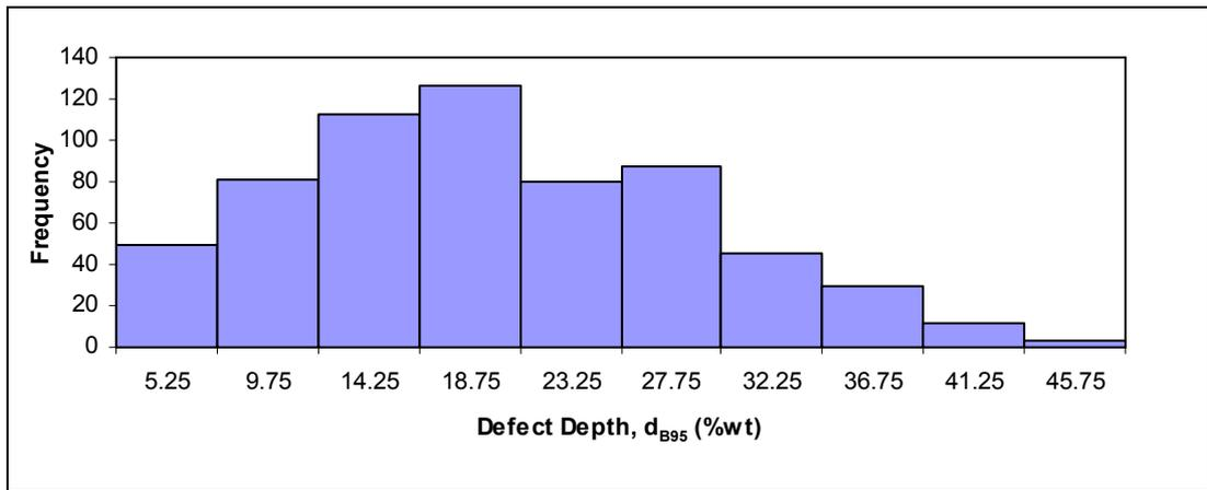
Figure 3.10: The histogram of corrosion depth,  $d_{B95}$  (*Pipeline B*)
