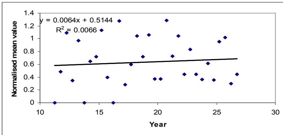
Figure 4.9: Linear regression analysis of mean depth and vessel age (rescaled data)
