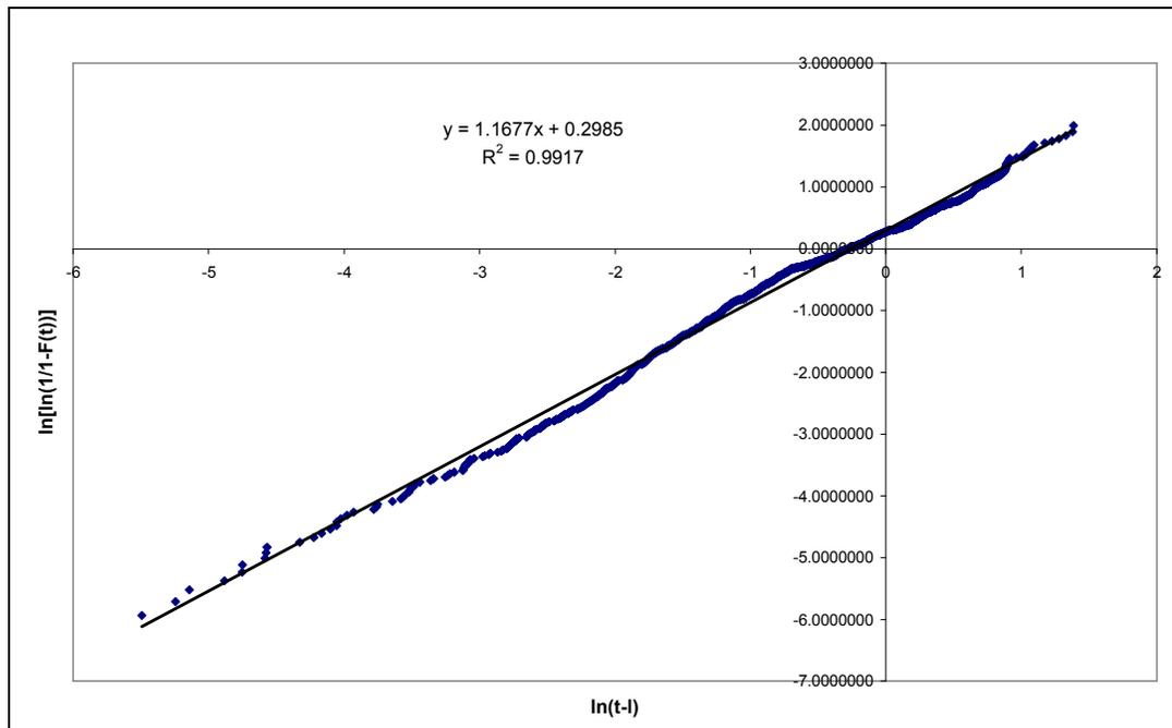
**Figure 4.7: Weibull probability plot of measured data (actual)**
