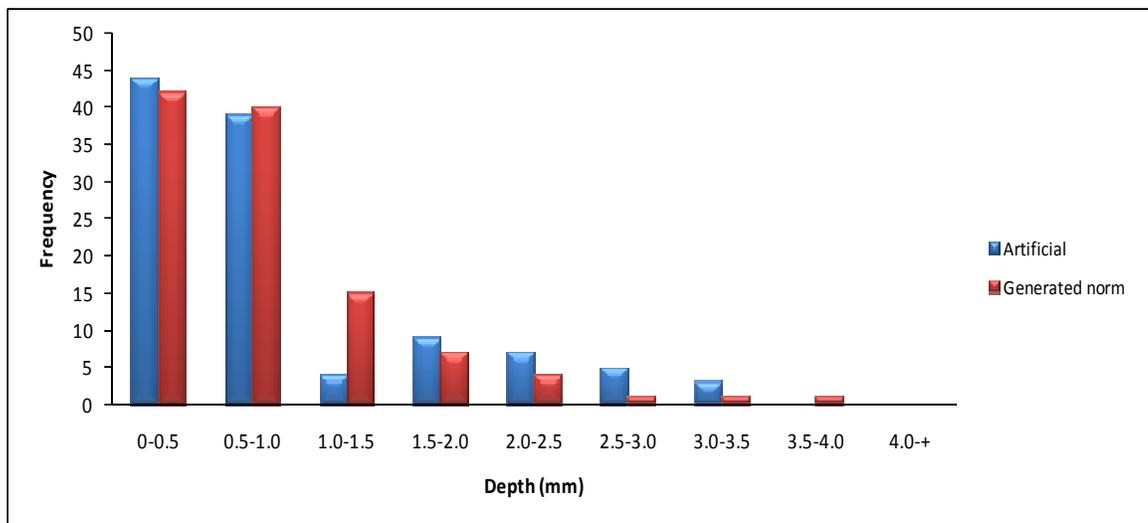
Figure 4.15: Comparison of predicted depth data to actual data for vessel age of 22-22.5 years old (RMSE of  $\pm 4.47$ )
