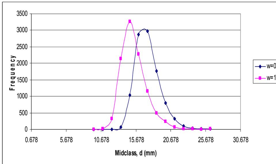
**Figure 3.25: Comparison of predicted extreme defect depth to actual depth based on extreme growth model and partial factor of 0 and 1 (*Pipeline B*)**
