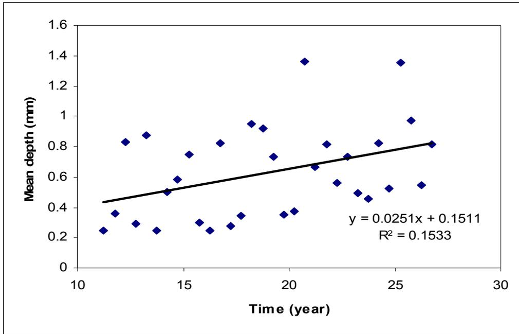
Figure 4.4: Linear regression analysis of mean value of defect depth and vessel age
