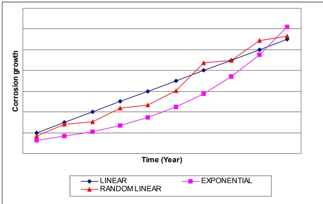
Figure 3.26: An illustration of three different patterns of corrosion growth
