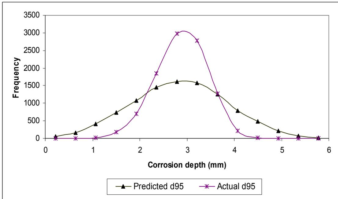
**Figure 3.20: Comparison result: Prediction of data from 1992 to 1995 using uncorrected corrosion growth rate (*Pipeline B*).**
