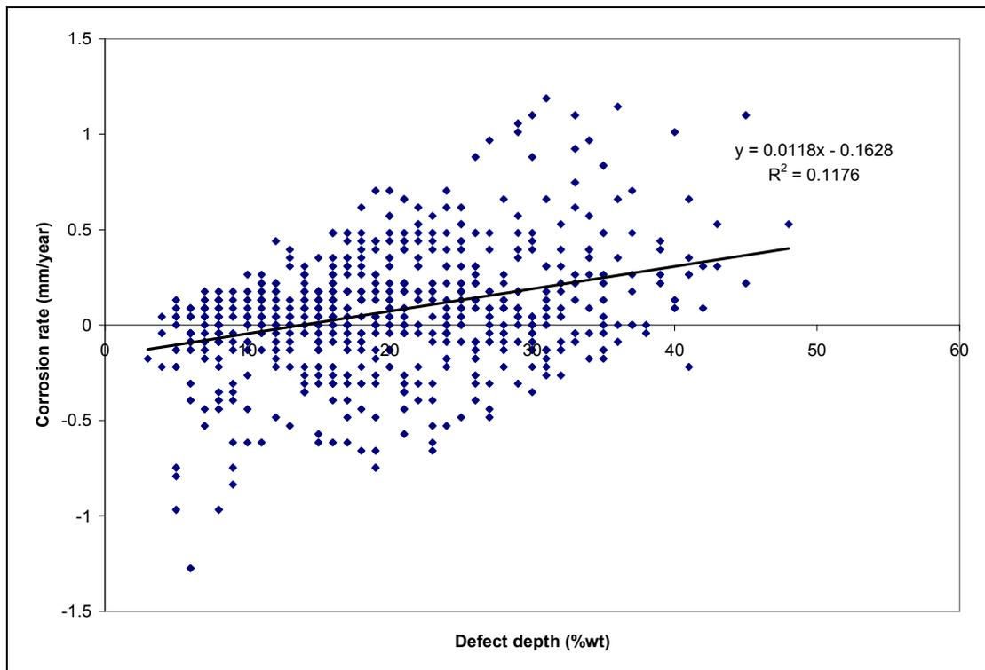
**Figure 3.7: Corrosion rate,  $CR_{B90-95}$  plotted against defect depth  $d_{B95}$  with linear regression line.**
