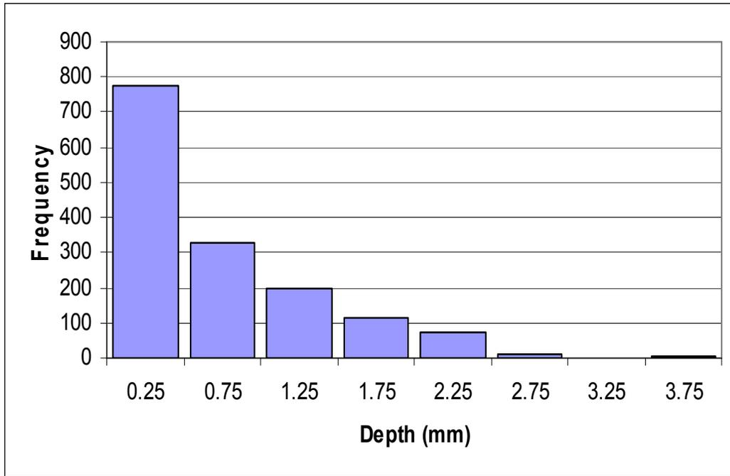
**Figure 4.6: Histogram of the whole set of corrosion depth**
