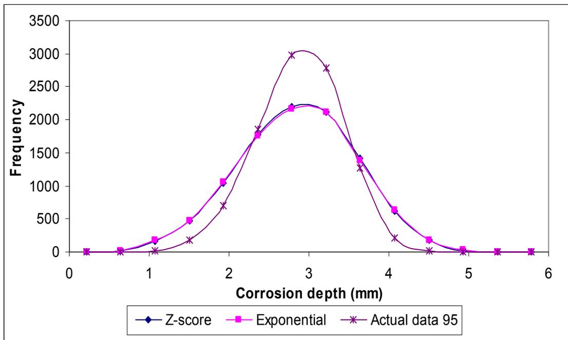
**Figure 3.21: Comparison result: Prediction of data from 1992 to 1995 using corrected corrosion growth rate (*Pipeline B*).**
