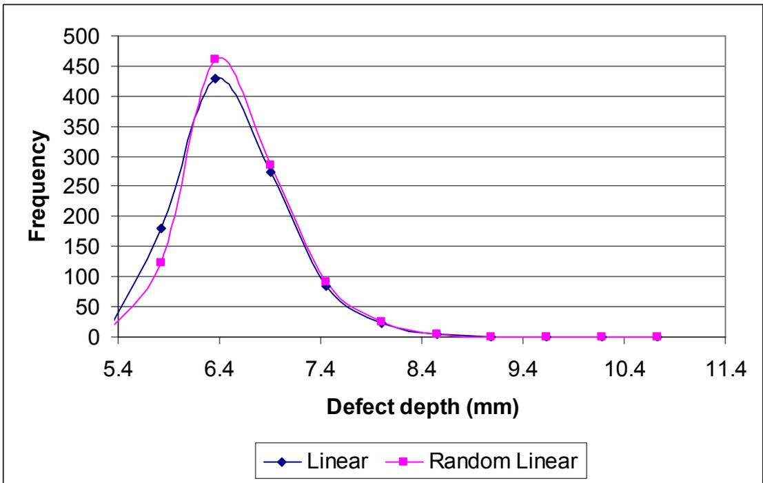
**Figure 3.30: Comparison of predicted corrosion depth to actual depth in year 1995 using linear and random models (*Pipeline A*)**
