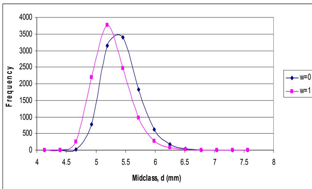
**Figure 3.23: Comparison of predicted extreme defect depth to actual depth based on extreme growth model and partial factor of 0 and 1 (Pipeline A)**
