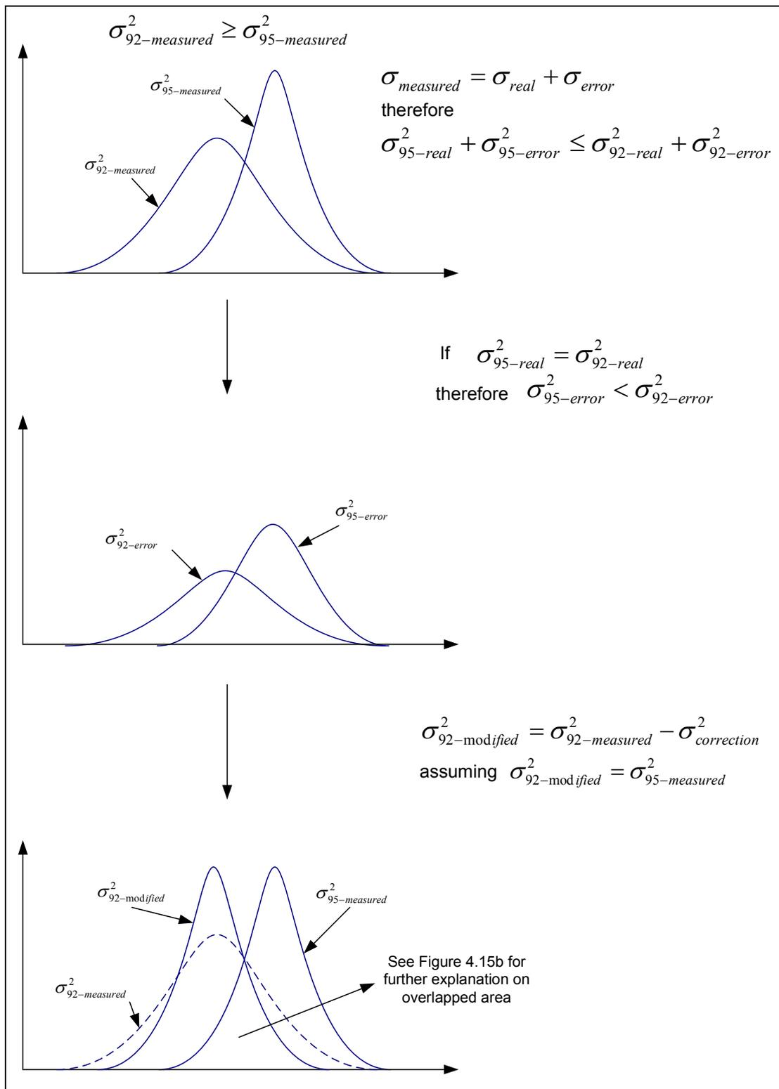
**Figure 3.15a: Illustration of modified corrosion rate.**
