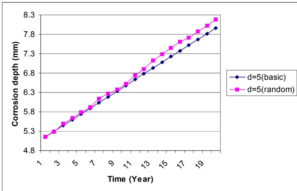
Figure 3.27: Linear prediction of corrosion defects by using basic and random linear models (d=5mm)
