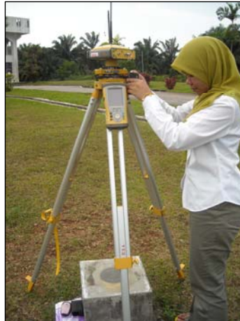
Figure 5.16: Base Station at UTM 01
