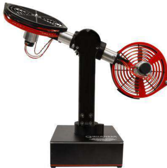
Figure 1: A 2-DOF helicopter model (Abdelkader and Kais, 2019)
