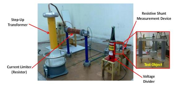
Figure 3.8 Experimental Setup of Total Leakage Current Measurement
