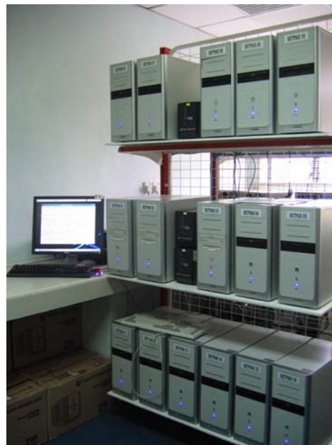
Figure 2. Cluster of parallel-computing set up for VASP calculation.
