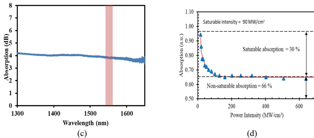
**Figure 1.** (a) The image of thin film with approximately 3.3 cm diameter, (b) EDS spectrum, (c) linear absorption spectrum, and (d) nonlinear absorption spectrum of  $\text{Sm}_2\text{O}_3$ .
