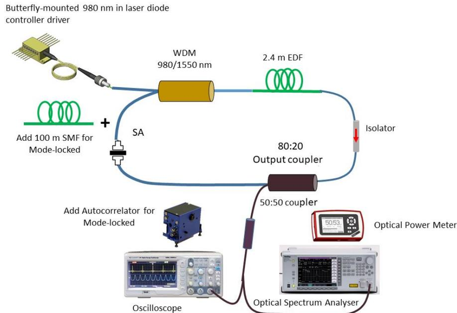
Figure 2. Experimental setup for picosecond mode-locking generation in an EDFL cavity.
