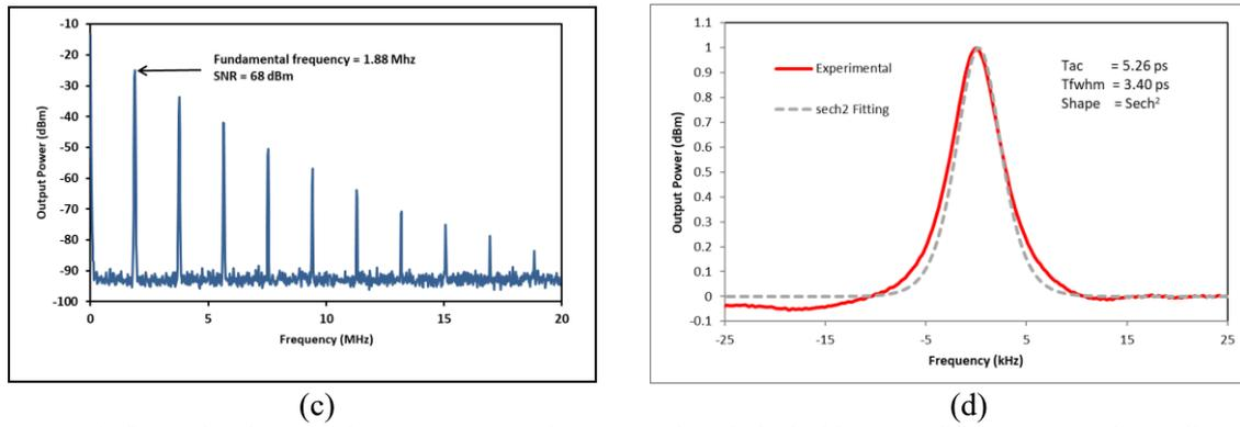
**Figure 3.** Spectral and temporal performances of the generated mode-locked laser; (a) OSA spectrum, (b) oscilloscope spectrum, (c) radio frequency spectrum, and (d) autocorrelator trace.
