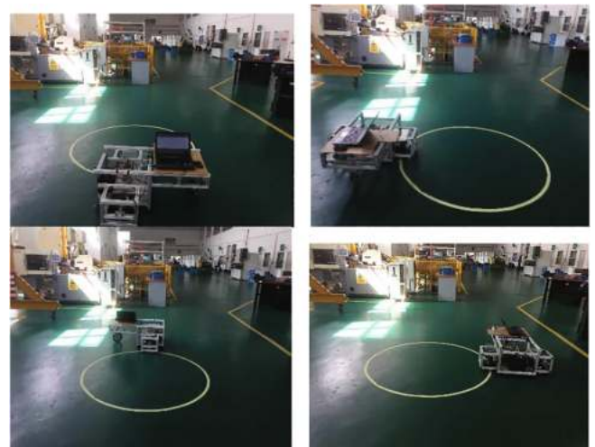
Fig. 21. A sequence of WMR movements on a circular path.
