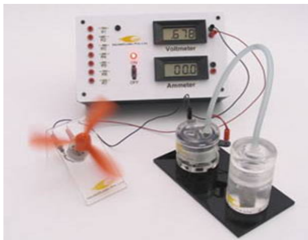
Figure 9: Model fuel cell run on our functionalized nanocomposite proton exchange membrane.
