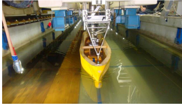
Fig. 7. LNG carrier model test in near bank and shallow water conditions.
